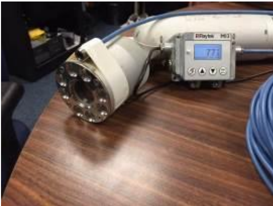
Figure 1-51. IR sensor attached to the inspection camera.
