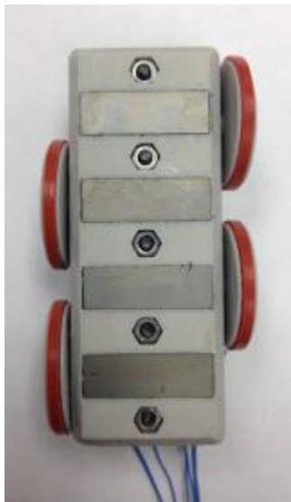
Figure 1-29. The assembled inspection tool using the 3D printed clamp and fasteners.
