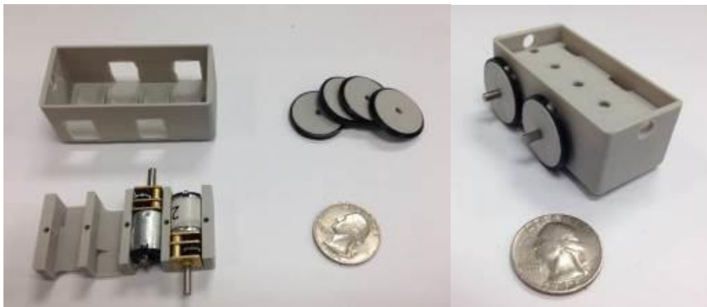
Figure 1-34. 3D printed components for inspection tool with micro metal gear DC motors and the assembly.
