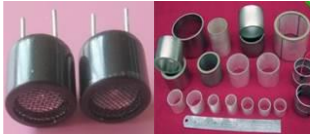
Figure 1-57. Piezo-electric micro-transducer elements [2].
