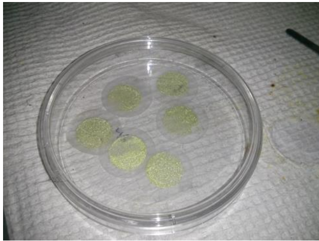
Figure 2-3. 0.45 \mu m filters with autunite particles.
