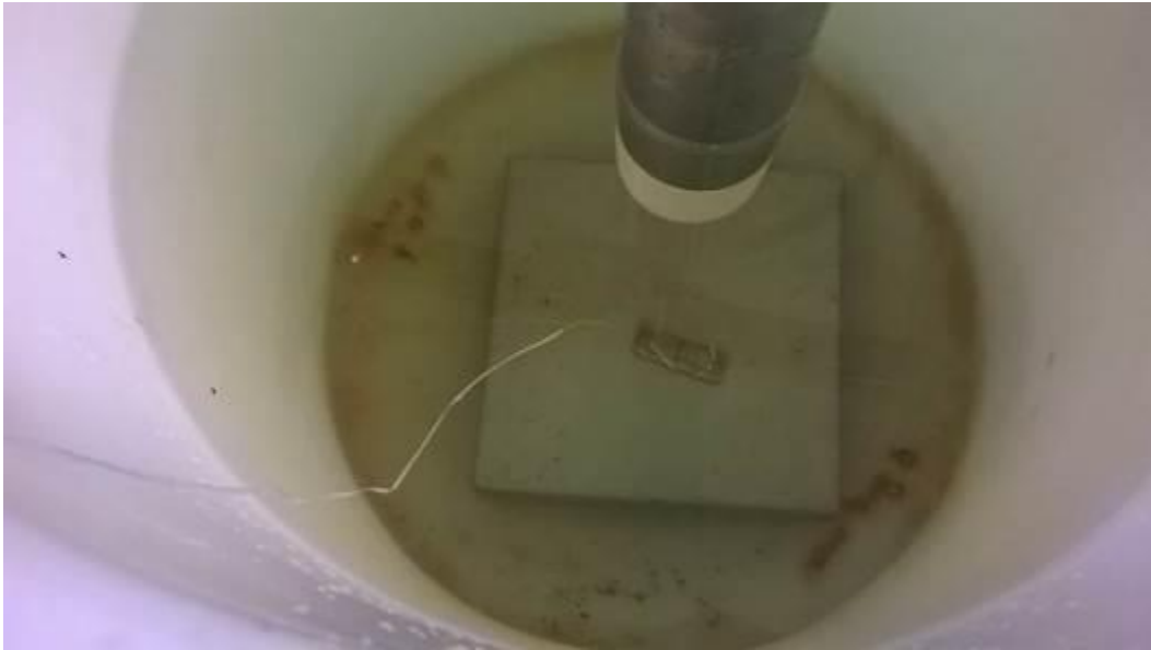
Figure 1-24. Test setup in small tank with 3D sonar and small stacked metal plates.
