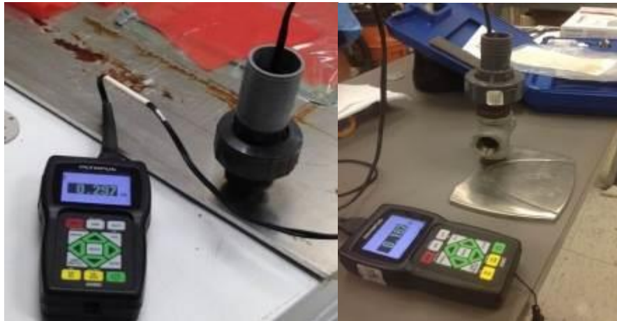
Figure 1-54. Experimental setup with loads on the sensor [aluminum (left) and stainless steel (right) test plates].
