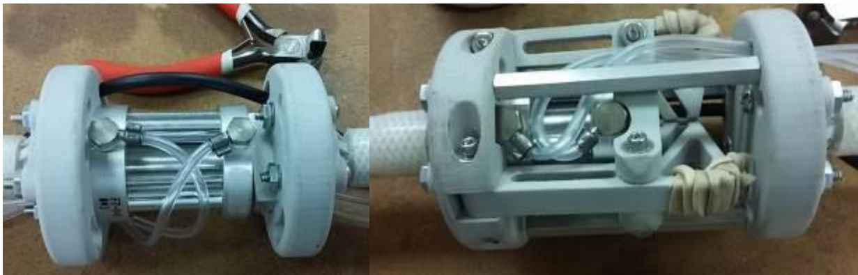
Figure 1-36. Metal clamps installed in the crawler pneumatic barbed connectors.
