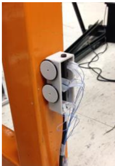
Figure 1-31. Inspection tool maneuvering up a vertical beam.
