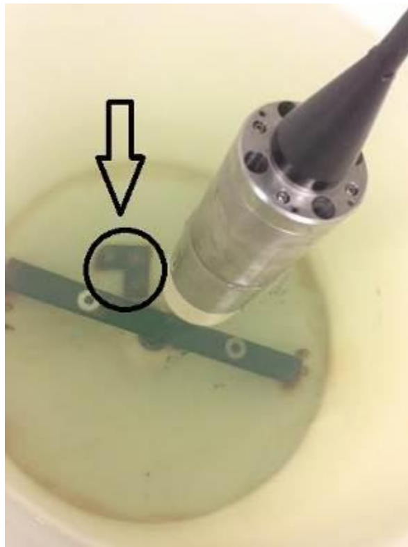
Figure 1-20. Setup to test the ability of the 3-D sonar to image a 6-mm thick metal piece.
