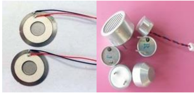
Figure 1-56. Piezo-electric micro-transducer elements [2].
