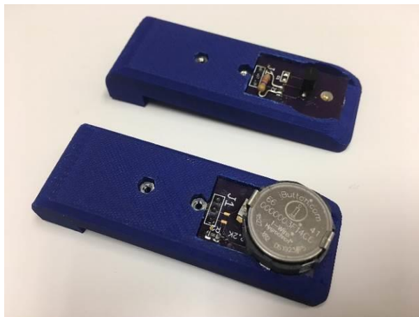
Figure 1-11. Sensor hoops populated with both the temperature and iButton sensors.
