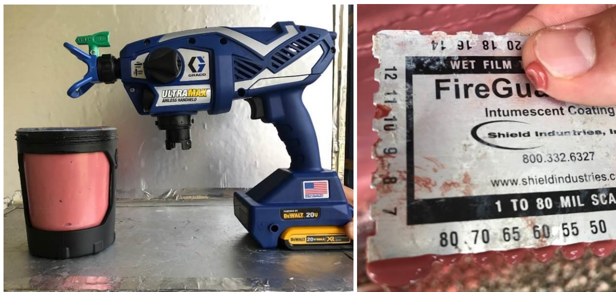
Figure 3-10. Airless sprayer (left) and manual film thickness gauge (right).
