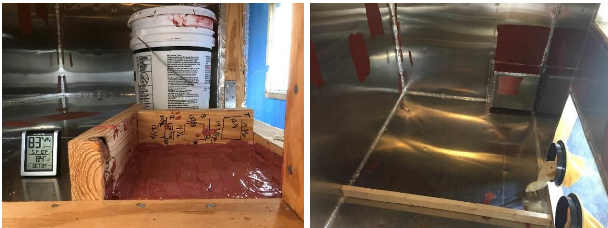
Figure 3-6. Small scale test of a slow pour technique using intumescent coatings (left) and preparing for full-scale demo of slow pour application method for horizontal / floor surfaces in hot cell (right).
