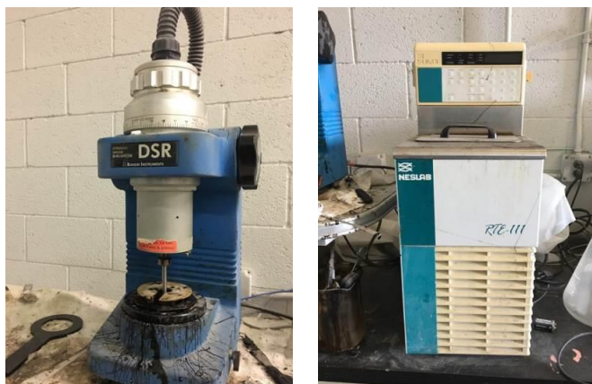
Figure 1-3. Dynamic shear rheometer (DSR) available at FIU (left) and water cooling bath (right).
