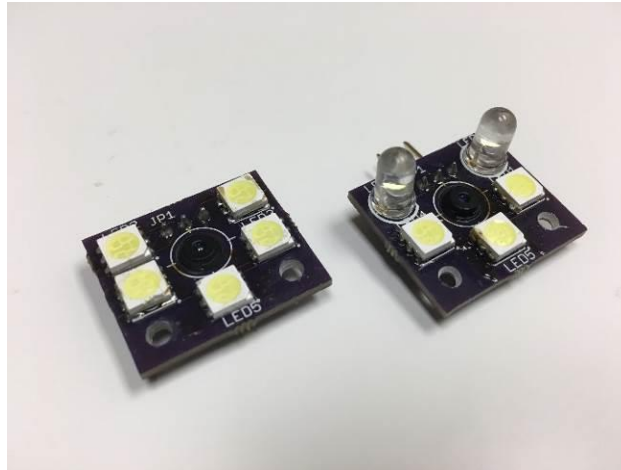
Figure 1-12. All patch LED lights on the left, mixed LED lights on the right for the lighting source of the mini inspection tool.
