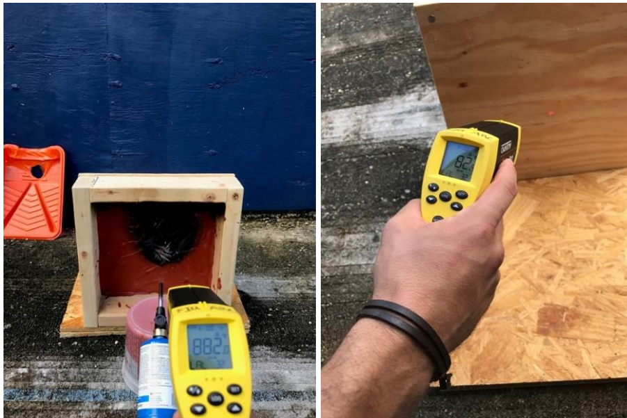
Figure 3-9. Fire testing a 18"x18" wooden test coupon after applying IC to 1/8" thickness using a slow pour method.
