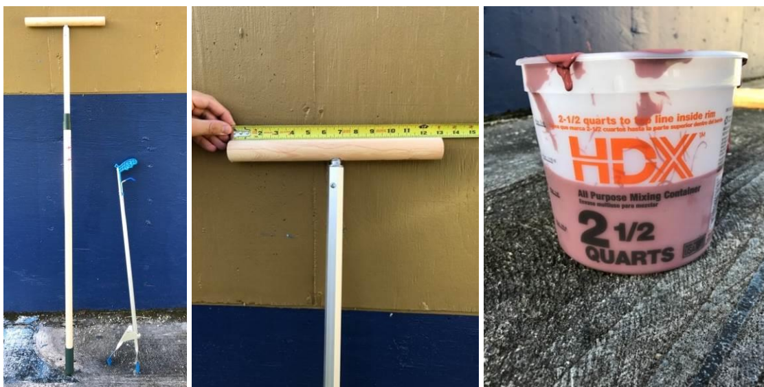
Figure 3-7. Tools used for slow pour method to apply IC to hot cell floor.
