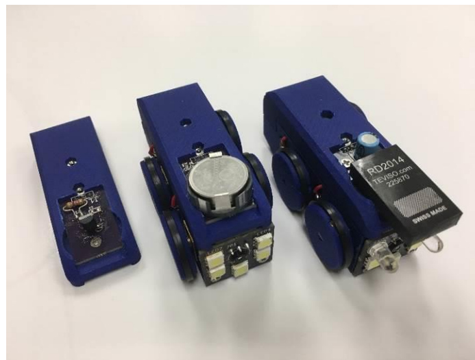
Figure 1-13. Temperature sensor hood (left), inspection tool fitted with iButton (humidity and temperature) sensor (middle), and inspection tool fitted with RD2014 Radiation sensor (right). The sensor hoods share a common electrical and communication interfaces.
