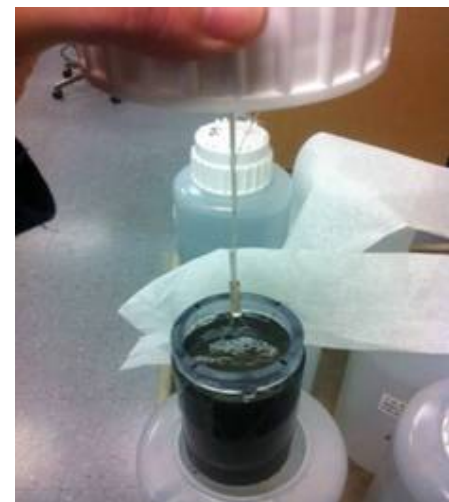
3" x 6" cylinder salt stone sample in leaching process
