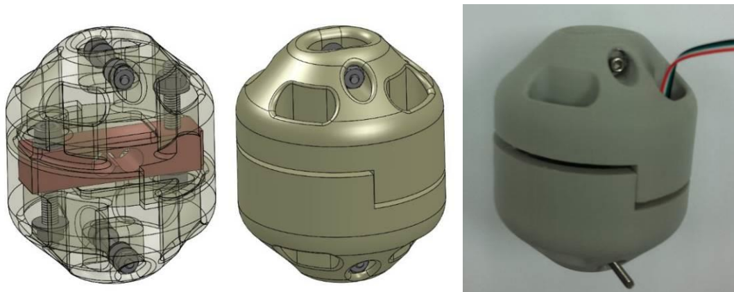
Figure 1-31. 100 lbs tether load cell.
