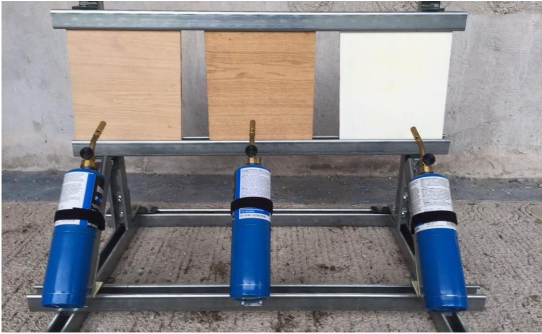
Figure 3-1. ARC constructed a platform that would allow the safe execution of a series of proof-of-principle experiments. The far left panel is wood only, the middle panel is wood with a leading industry fixative, and the far right panel is wood with a leading industry fixative layered with an intumescent coating.
