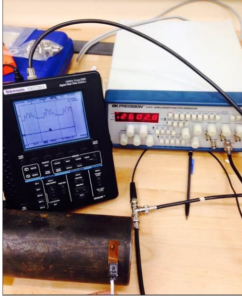
Figure 1-47. Smart sensor placed on a pipe.
