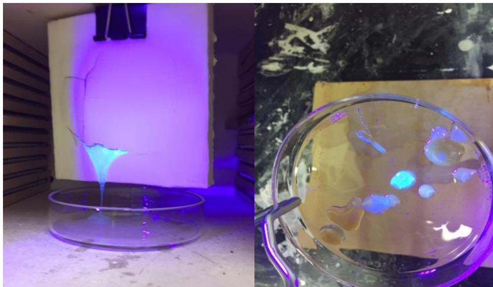
Figure 3-6. Fixative with GloGerm flowing through fissure in intumescent coating when exposed to heat at 400-500° F (left); image of petri dish showing fluorescing GloGerm.
