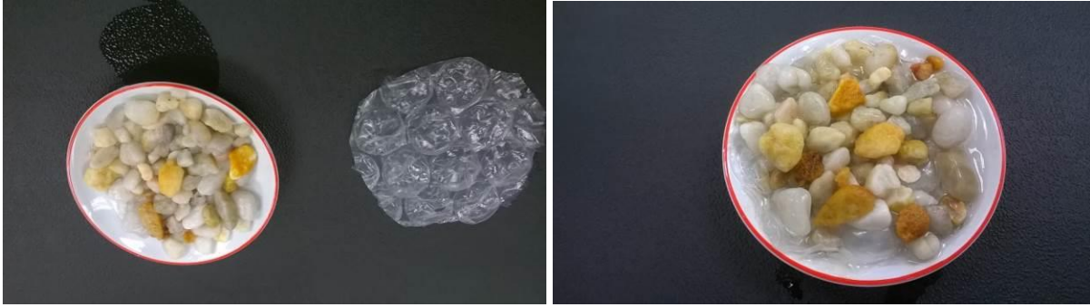
Figure 1-11. Plate of pebbles for sonar imaging and bubble wrap (left) and bubble wrap inserted under pebbles (right).
