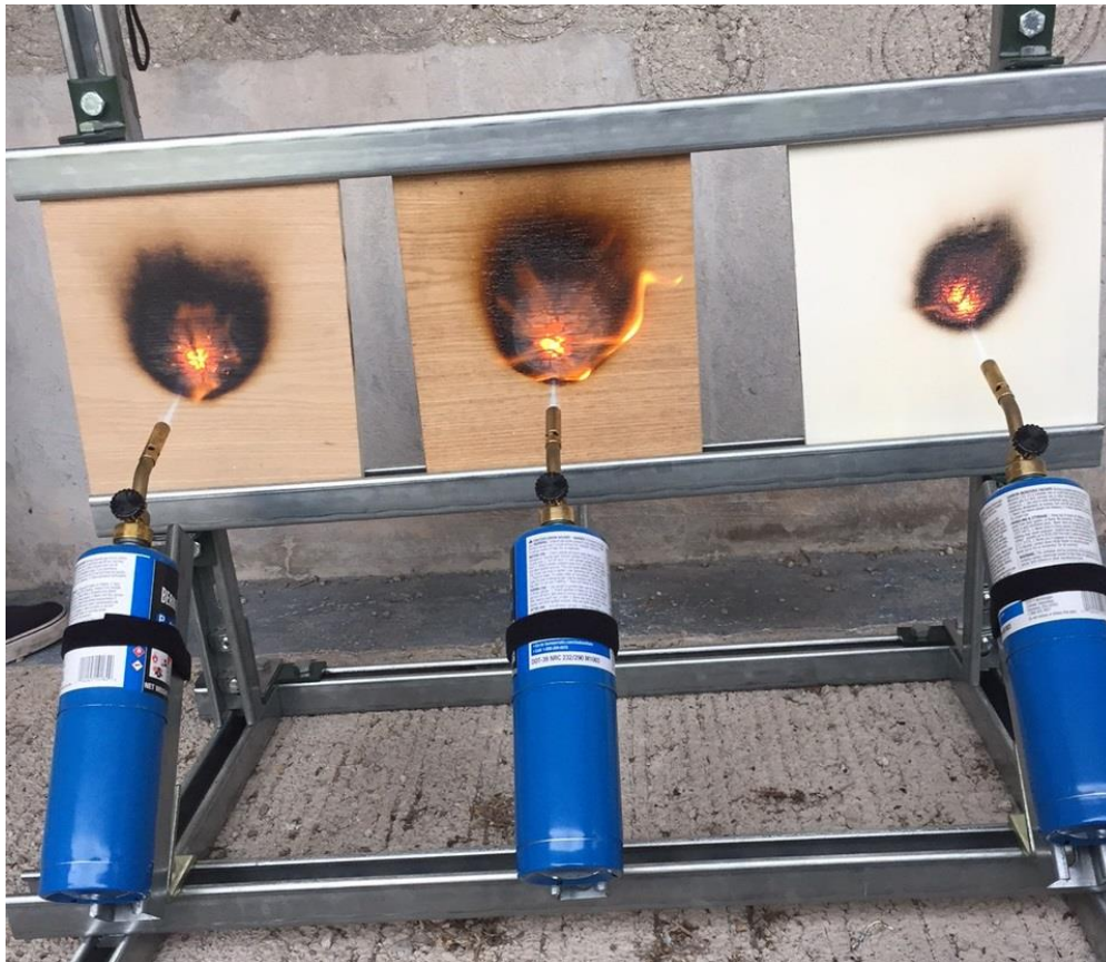
Figure 3-2. At the 2-minute mark, both the left and middle panels began to show significant degradation and burn through while the right panel began to develop a thickening char from the expanding intumescent coating.
