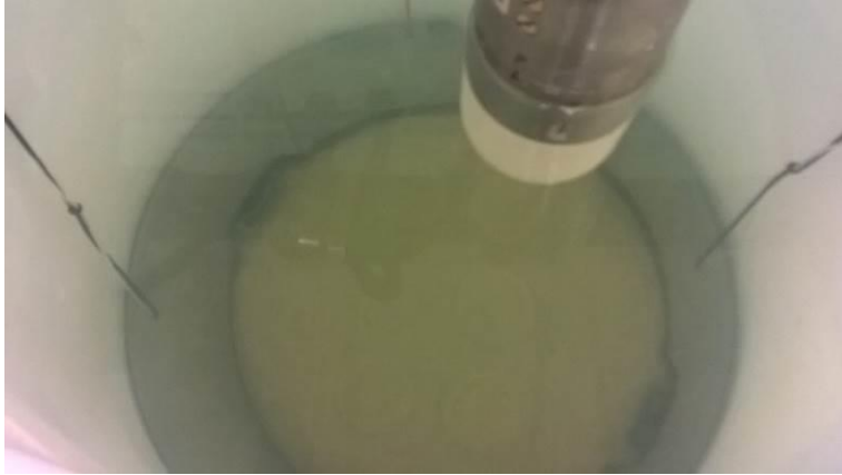
Figure 1-19. Photograph of plastic lid filled with sand on an aluminum plate on the tank bottom. The 3D sonar can be seen in the center top of the photograph.
