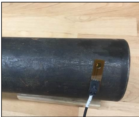
Figure 1-44. Smart sensor placed on a pipe.
