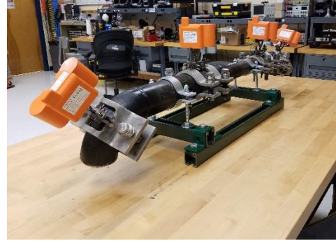
Figure 1-39. Permasense sensor system: on pipe section (left) and detailed view (right).
