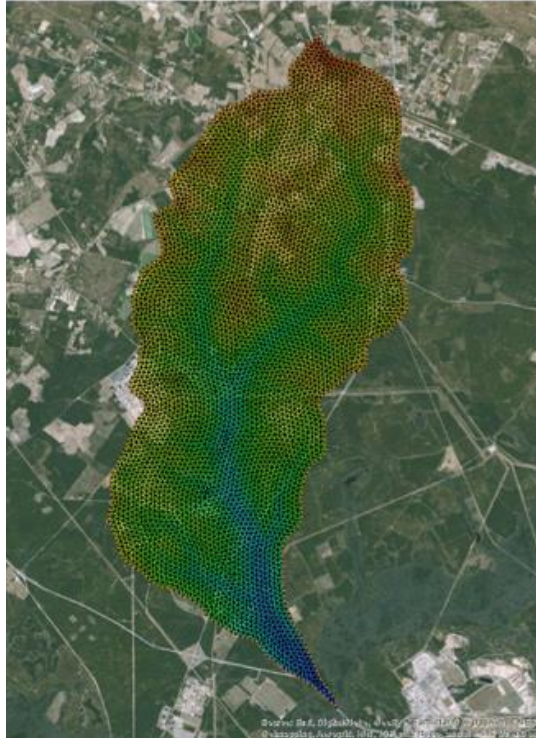
Figure 2-14. Preliminary Unstructured mesh developed on Tims Branch Watershed as part of the implementation of the alternative hydrologic flow and transport model.
