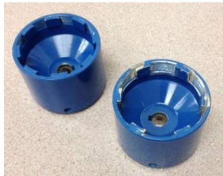
Figure 1-42. Old (top) and new (bottom) drive magnets.
