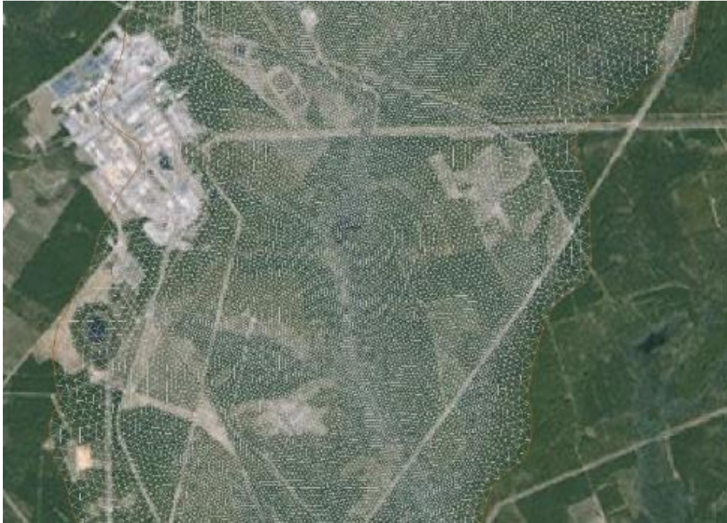
Figure 2-16. Detail of the hydrologic model refined mesh. Note that the mesh has higher resolution (smaller cells) on areas of more interest, while cells are larger along the boundaries.
