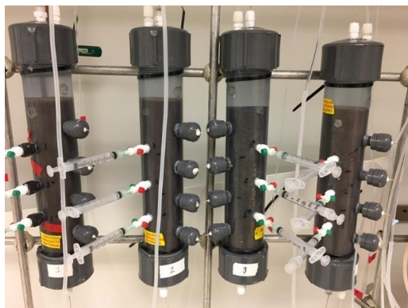
Figure 2-9. Experimental columns with syringe and needles inserted in the sampling ports.
