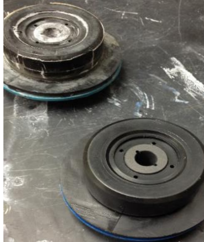
Figure 1-41. Old (top) and new (bottom) pump impellers.
