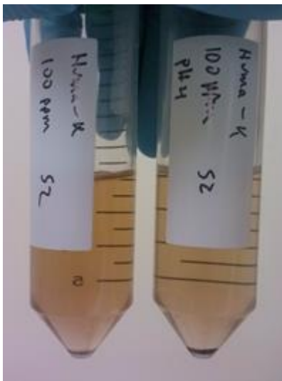
Figure 2-35. Comparison of two Huma-K samples (concentration 100 ppm) at two different pH values
