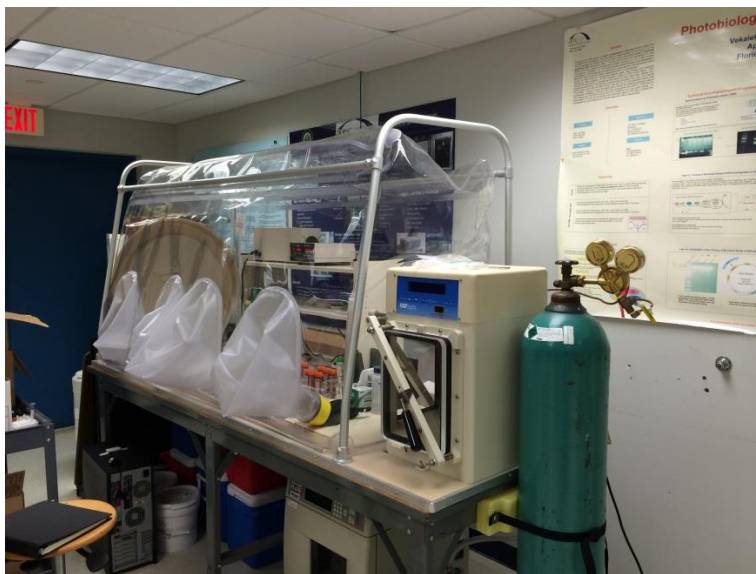
Figure 2-11. Anaerobic chamber used for the microcosm experiment
