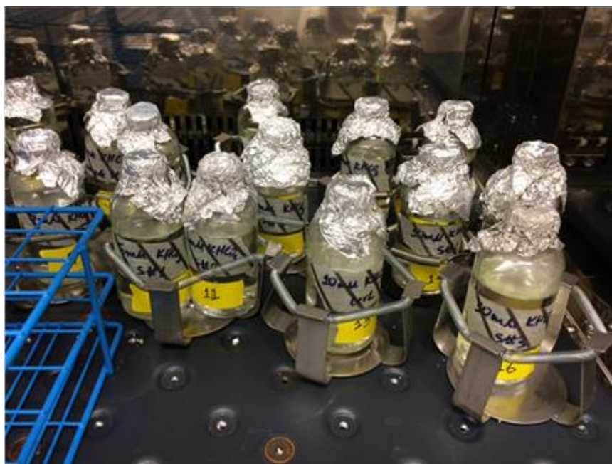
Figure 2-5. Control and experimental bottles prepared for the bioleaching experiment.
