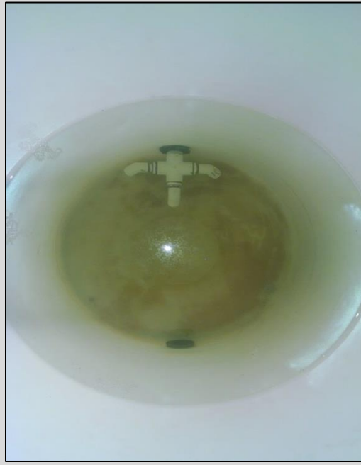
Figure 1-3. Object to be imaged (a section of unistrut or U-channel) (left). Test tank from above showing 3 inlet nozzles and the outlet return (right).
