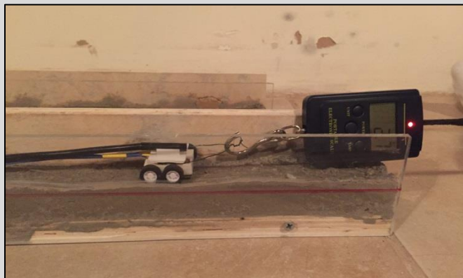
Figure 1-8. Pull force tests in the mock-up of the channel.
