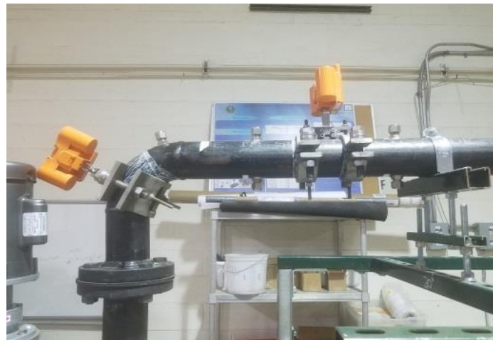
Coupons on the pipe loop
