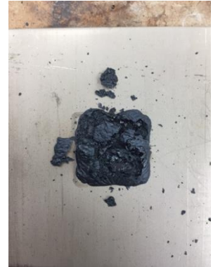
Finish: significant mass loss, discoloration, desiccation, cracking, and flaking.
