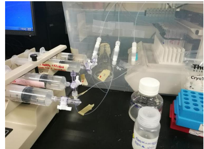
Mini-column experiment with four syringes connected to four mini.
