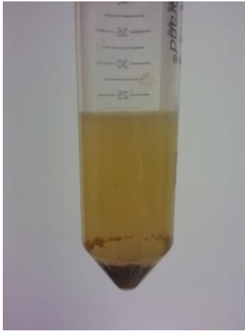
Centrifuge tube with amended sediment and uranium
