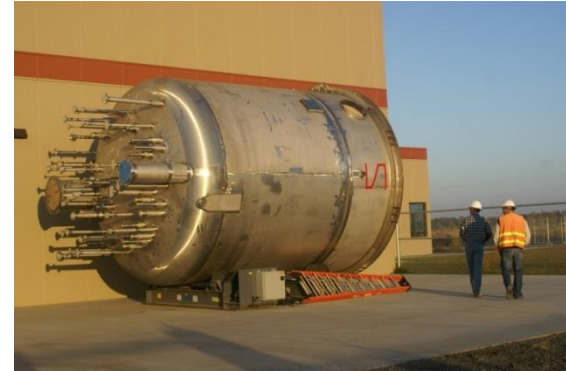
14-ft-diameter vessel to test PJMs
