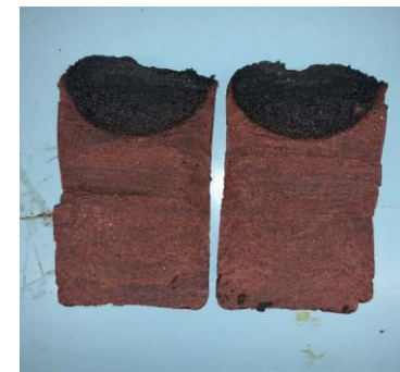
Intumescent Foam Sample (cut in half) Post Direct Flame Test
