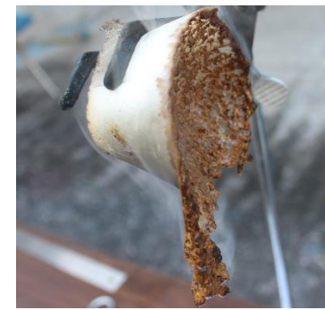
Fire Rated Foam Sample Post Direct Flame Test
