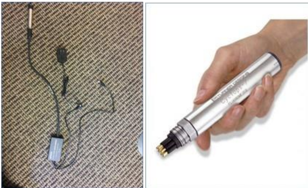
Figure 66. Turner Designs Cyclops 7-F Turbidity Sensor with Explorer adapter.
