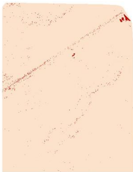
Figure 116. Output of subtracted rasters of ERGBVI with threshold values of -0.690367 and -0.558956 highlighting areas of greatest variation between each DEM in red.
