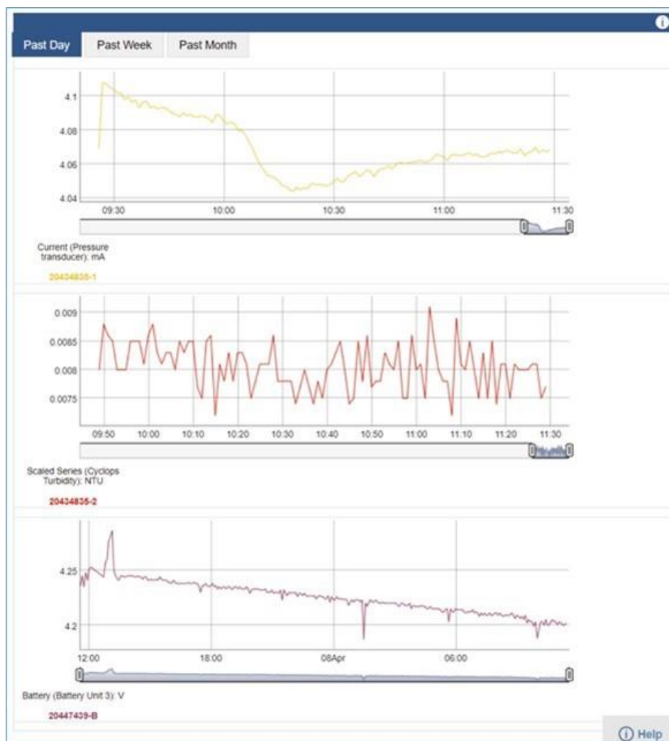
Figure 72. Successful integration of the HOBO RX3000 with the STEVENS pressure transducer and Cyclops turbidity sensor using the HOBOLink portal.
