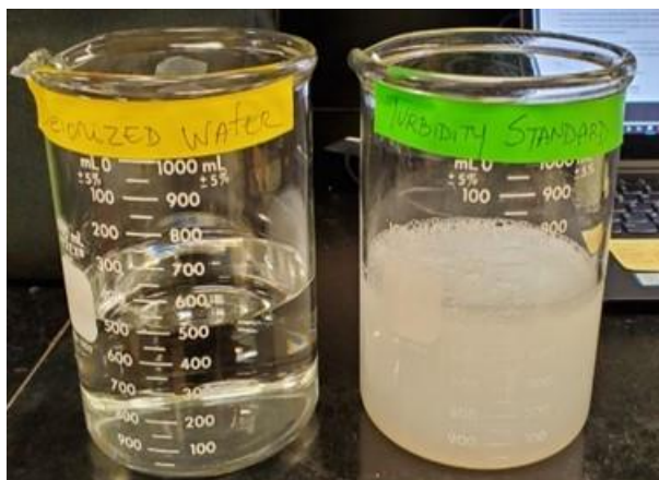
Figure 77. Calibration of Cyclops turbidity sensor using integrated EXPLORER software. The calibration was done using deionized water and a calibration standard of 1000 NTUs.
