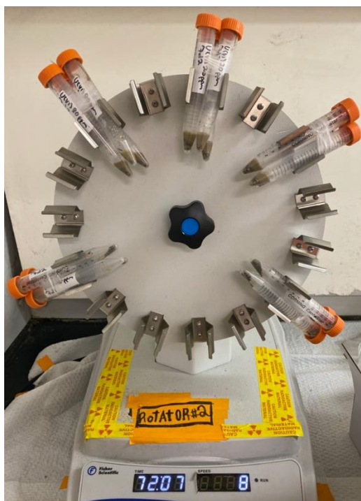
Figure 16. Sediment samples in an end-over-end tube revolver at 8 rpm.
