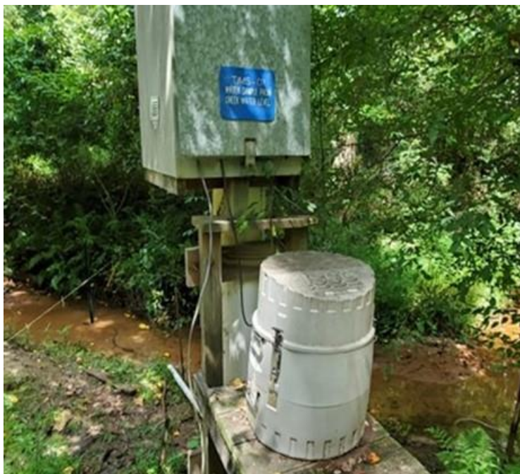
Figure 78. ISCO autosampler located in Tims Branch near Road C.
