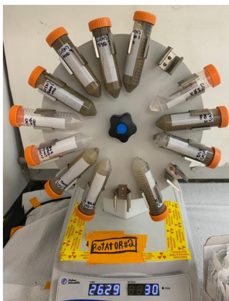
Figure 15. Sediment samples in an end-over-end tube revolver at 30 rpm.
