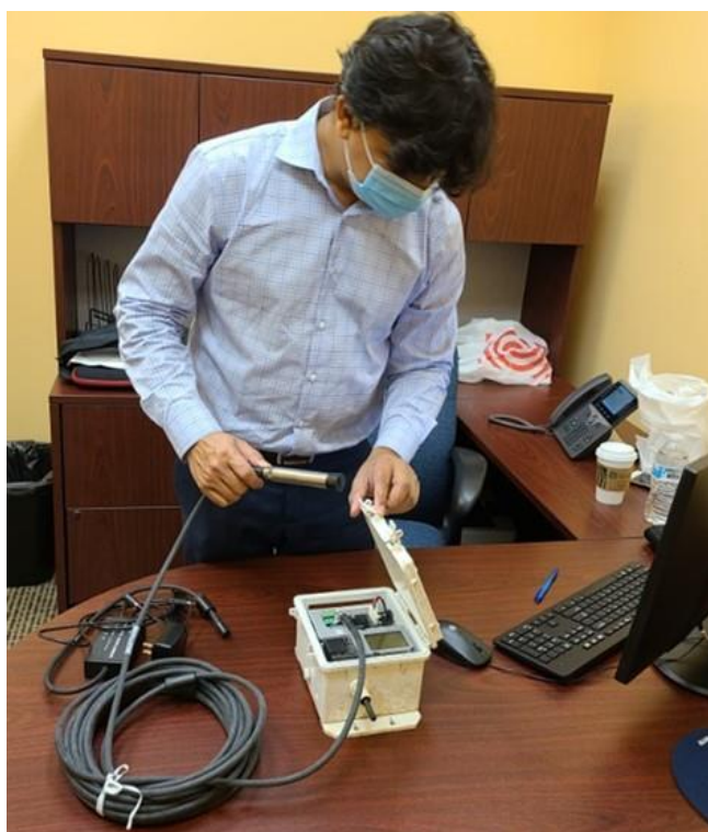
Figure 65. The Cyclops-7F submersible turbidity sensor being integrated into the HOBO RX3000 at FIU.
