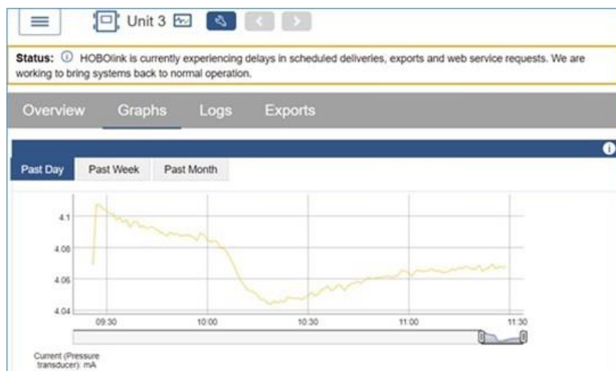
Figure 69. CHANNEL 1 - Unit 3 pressure transducer mA readings integrated using the HOBOLink portal.
