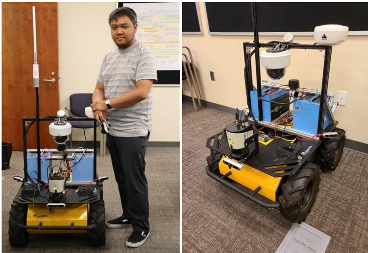
Figure 6. Clearpath Husky with new power and sensor package integrated.
