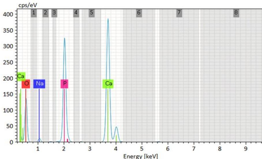
Figure 16. EDS element spectrum obtained for apatite formed during synthesis.
