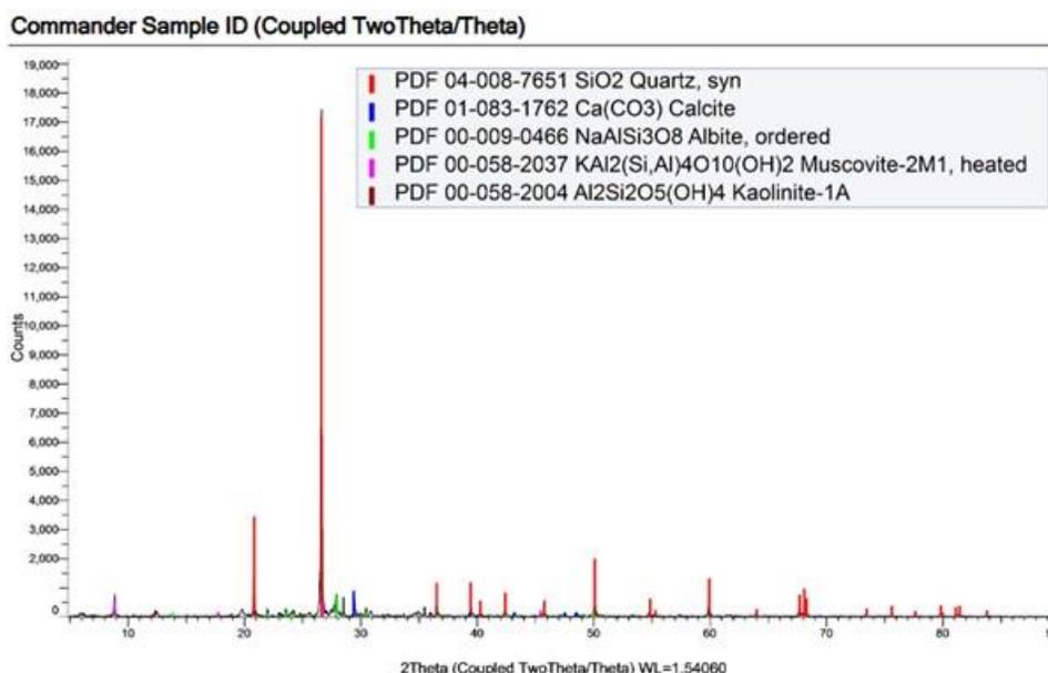
Figure 24. Matched XRD pattern for sediment sample from plot 4.
