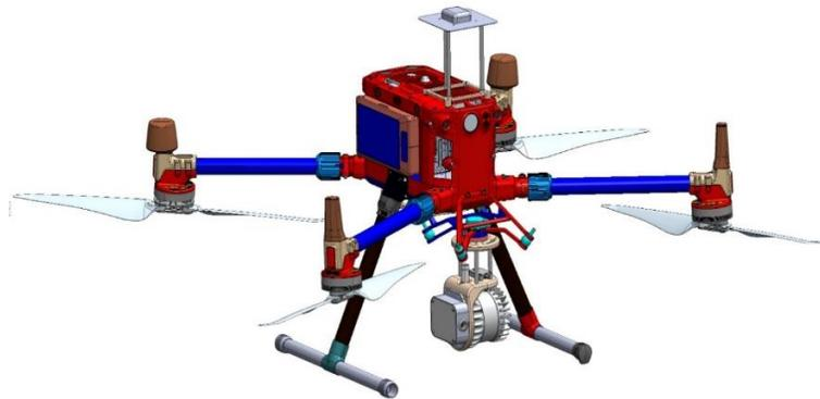
**Figure 44. CAD model of the Lidar module mounted below the DJI Matrice 300 RTK. This agnostic system includes a 3D printed mount with an embedded computer, auxiliary sensory, and supporting electronics.**
