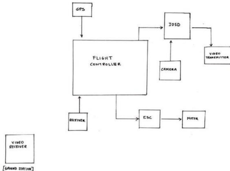
Figure 28. Typical main components in UAV systems.
