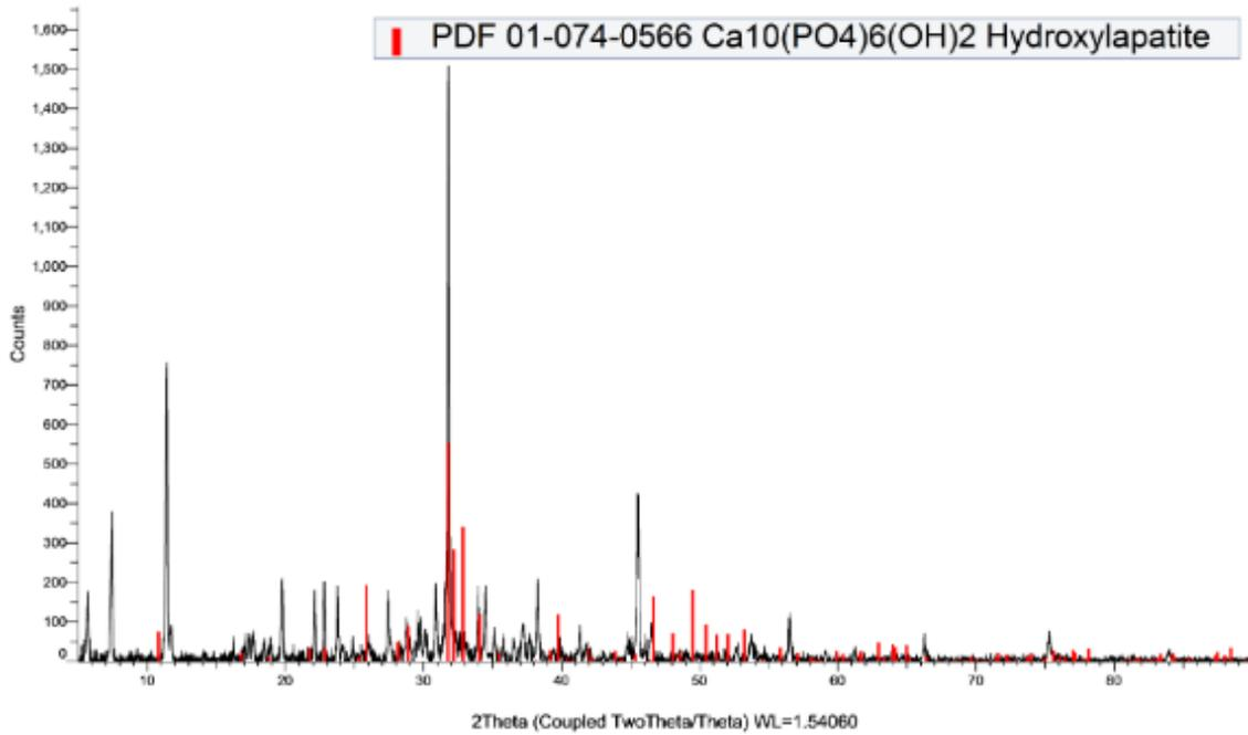
Figure 14. Scenario 4 XRD pattern matching with hydroxyapatite PDF.
