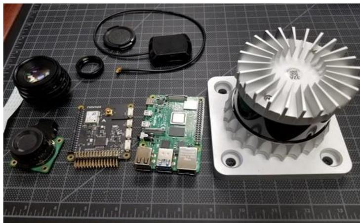
Figure 39. LiDAR system main components.
