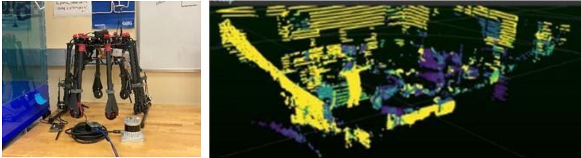
Figure 38. LiDAR and DJI S1000 UAV (left) and preliminary LiDAR testing (right).
