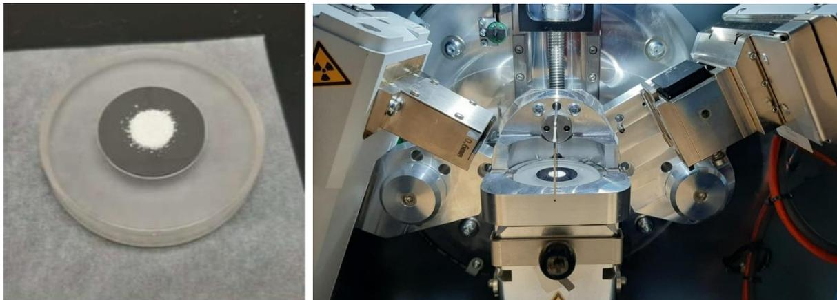
**Figure 6. Hydroxyapatite powder on sample holder prepared for XRD analysis.**
