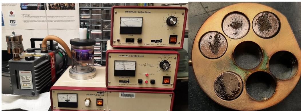
Figure 9. Instrument used to gold coat samples (left) and gold coated sediment samples (right).
