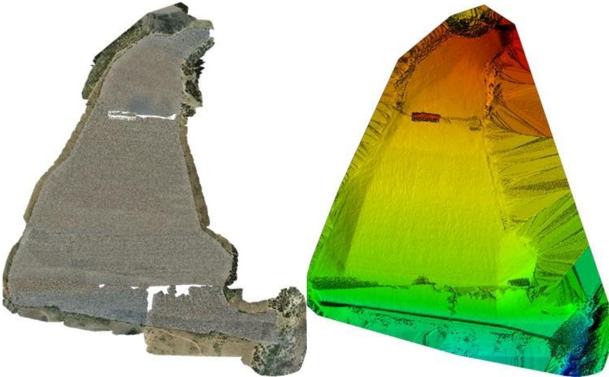
**Figure 48. Captured orthomosaic map (left) and digital elevation model (right) of Rifle Disposal Cell.**
