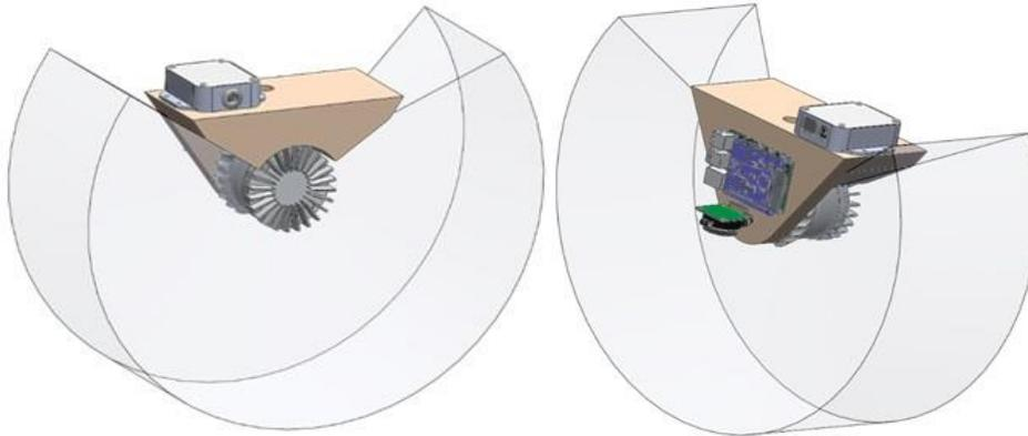
**Figure 41. FIU's remote sensing agnostic LiDAR package.**
