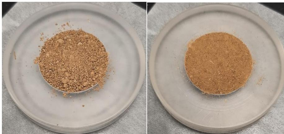
Figure 7. Plots 3 and 4 (left to right) sediment loaded onto sample holder prior to XRD analysis.
