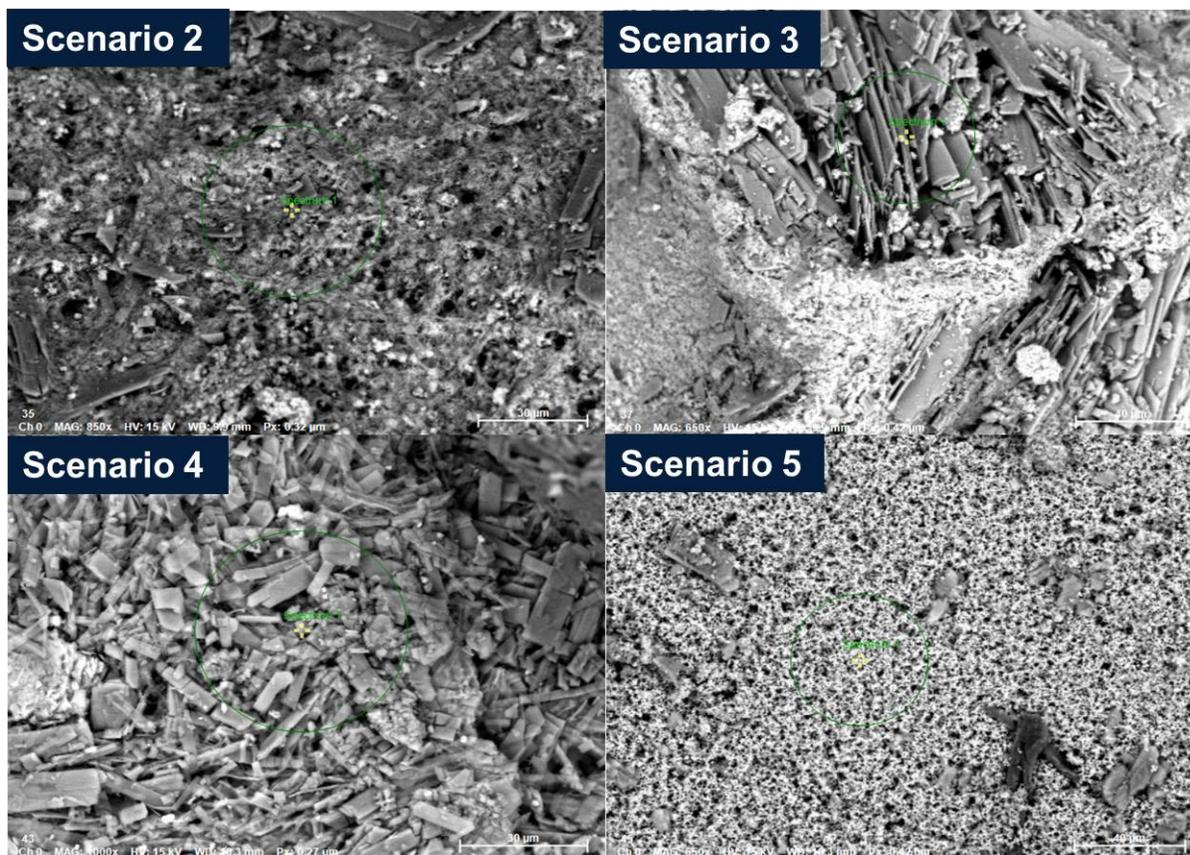
**Figure 17. SEM Images of hydroxyapatite formed during synthesis via different scenarios.**
