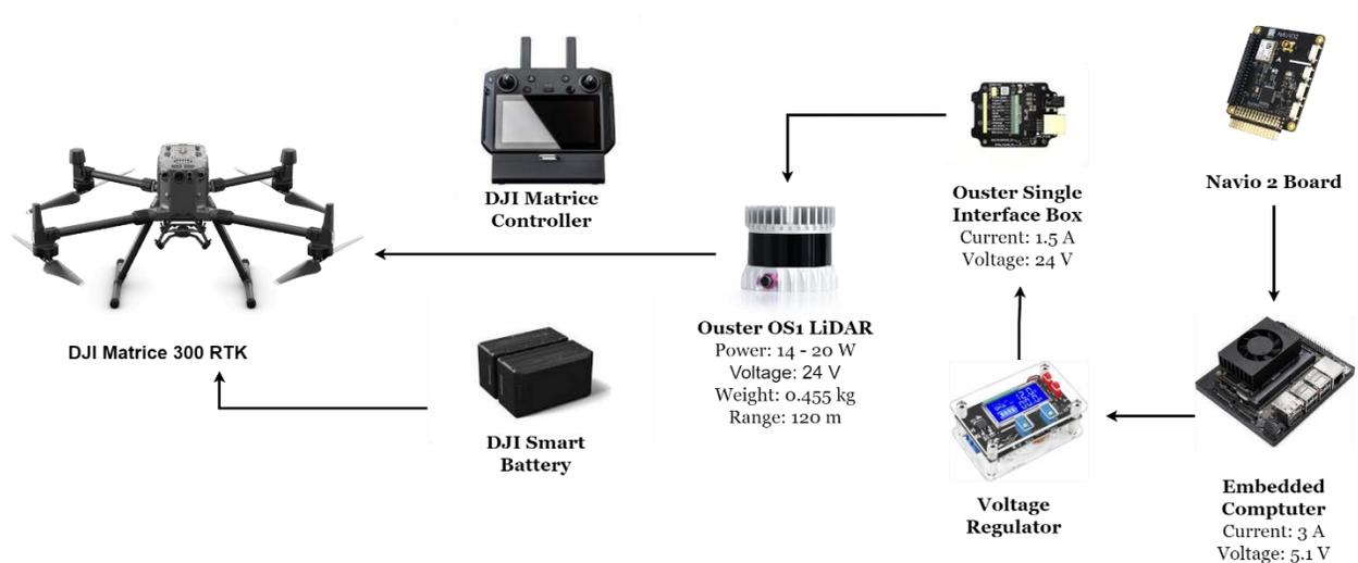
**Figure 45. Equipment used for LiDAR method**
