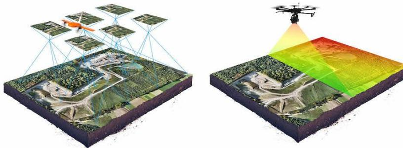
**Figure 30. UAV collecting aerial photographs from different locations along flight plan which provides digital elevation model when post processed. [3]**
