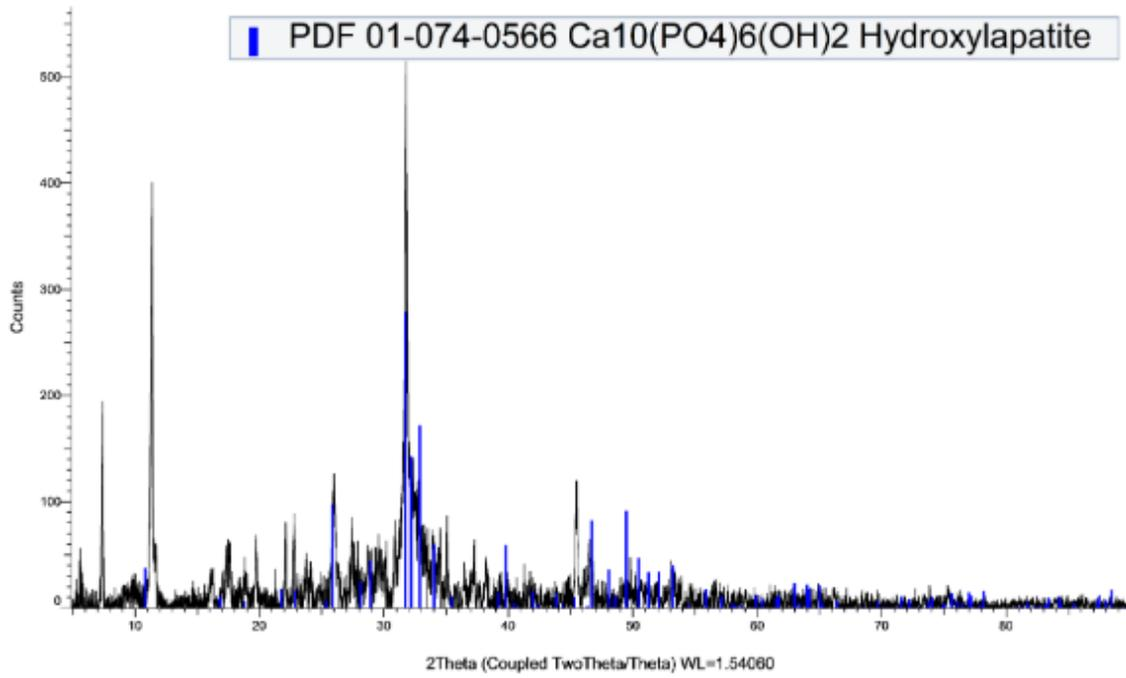
Figure 13. Scenario 3 XRD pattern matching with hydroxyapatite PDF.
