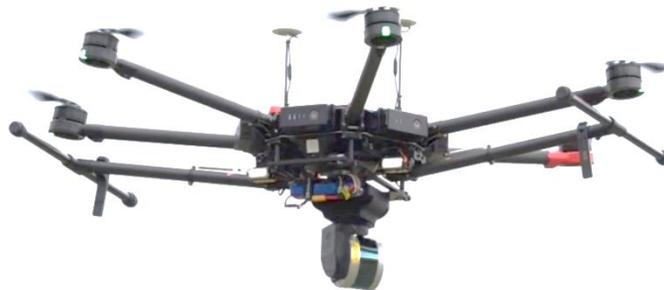
**Figure 36. FIU's UAV LiDAR mapping systems conceptual design.**
