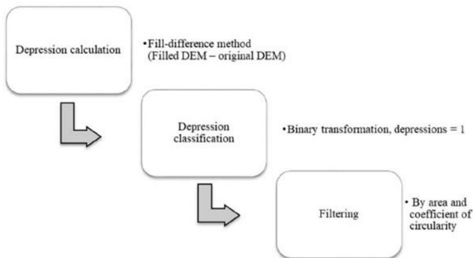
**Figure 50. Basic workflow to estimate depressions using DEMs.**
