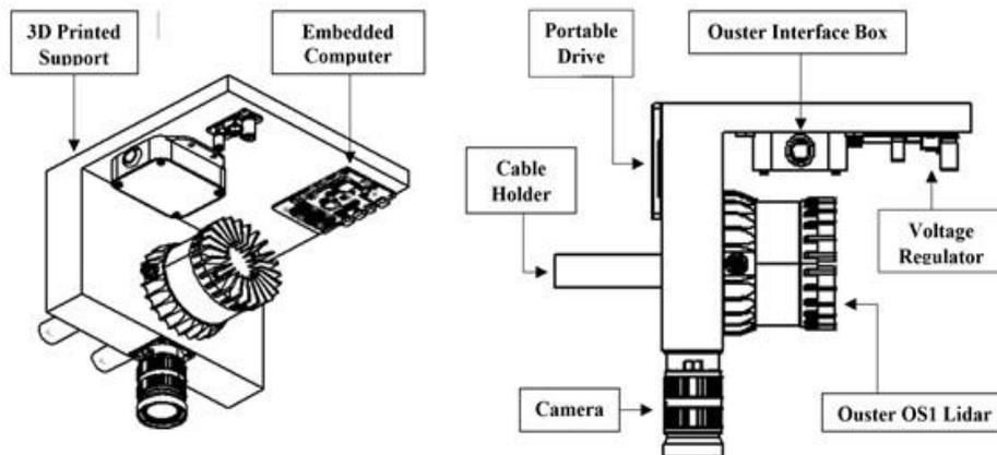
Figure 40. LiDAR mount conceptual design.
