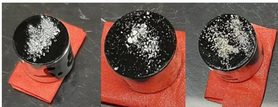
Figure 8. Dried HA Precipitate Prepared for SEM Analysis.
