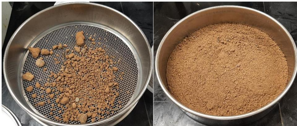
**Figure 4. Sediment sieved through 2-mm sieve.**
