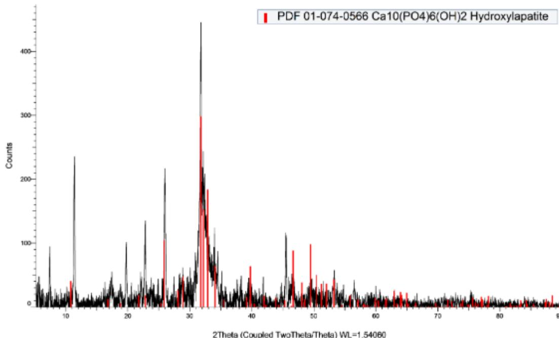
Figure 15. Scenario 5 XRD pattern matching with hydroxyapatite PDF.
