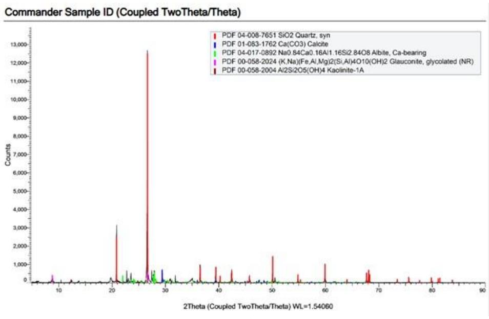
Figure 21. Matched XRD pattern for sediment sample from plot 1.
