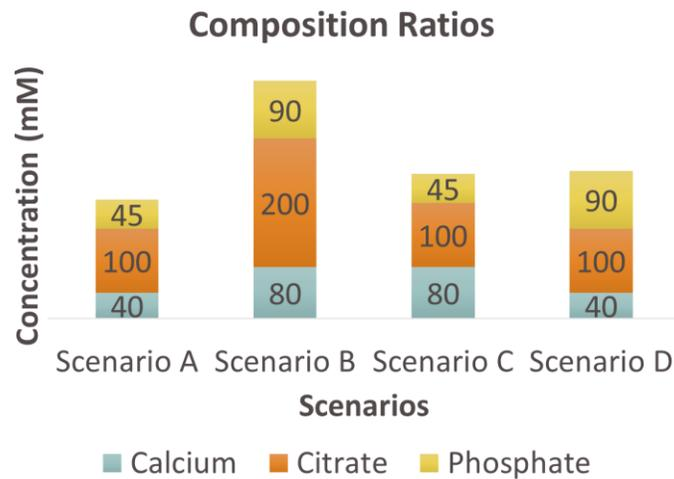
Figure 2. Composition of calcium, citrate and phosphate ratios tested during synthesis.
