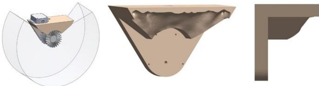
**Figure 43. Lidar bracket original design (left) and optimized (right).**
