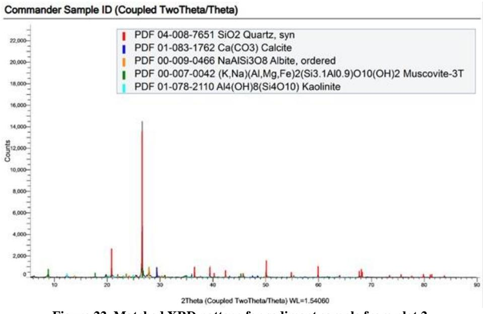
Figure 22. Matched XRD pattern for sediment sample from plot 2.
