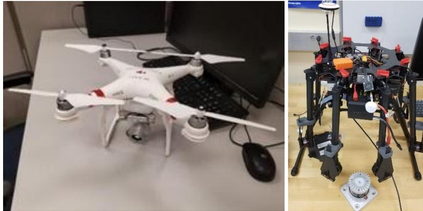
**Figure 26. FIU's photogrammetry (left) and LiDAR (right) mobile mapping systems.**
