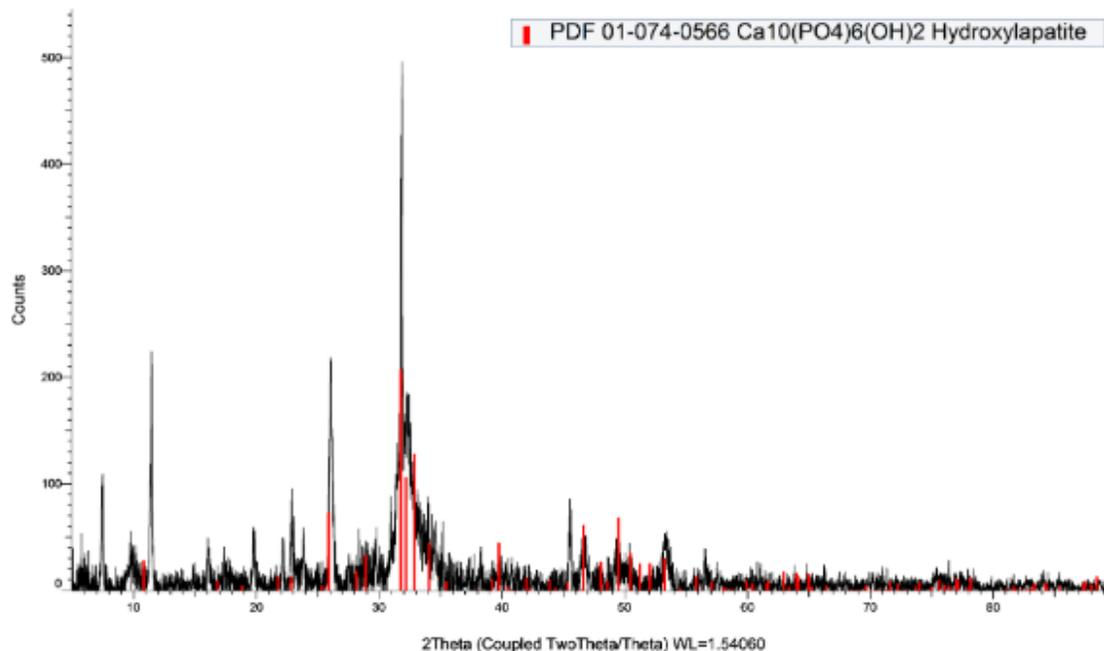
**Figure 12. Scenario 2 XRD pattern matching with hydroxyapatite PDF.**
