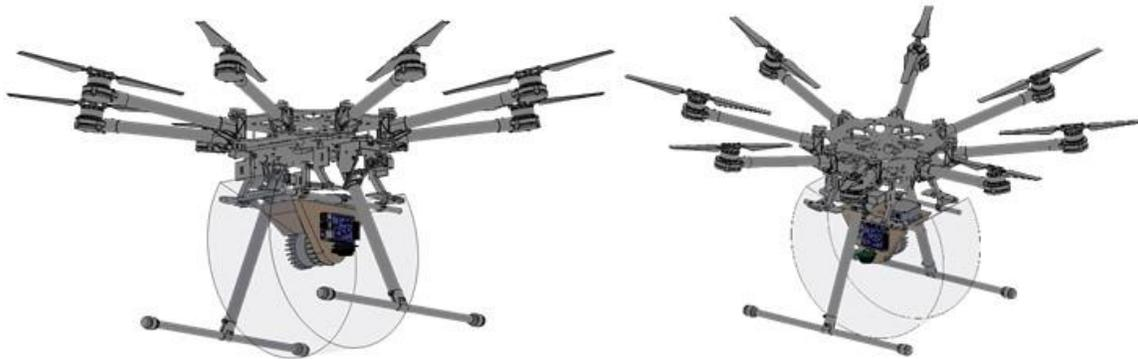
**Figure 42. LiDAR and aircraft integration preliminary design.**
