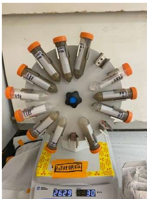
Figure 21. Sediment samples in an end-over-end tube revolver at 30 rpm
