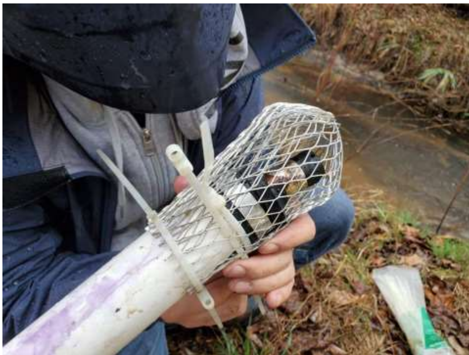
Figure 57. Protective wire mesh installed to prevent fouling of the water level sensor by sediment or debris.
