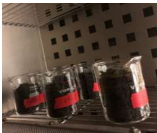
Figure 33. SRS soil samples being dried in the oven.
