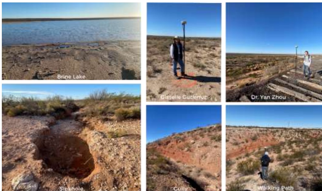
Figure 82. FIU team marking ground control points using a Trimble GPS receiver in Basin 6, taking note of surface hydrological features of interest including brine lakes, sinkholes, and gullies.
