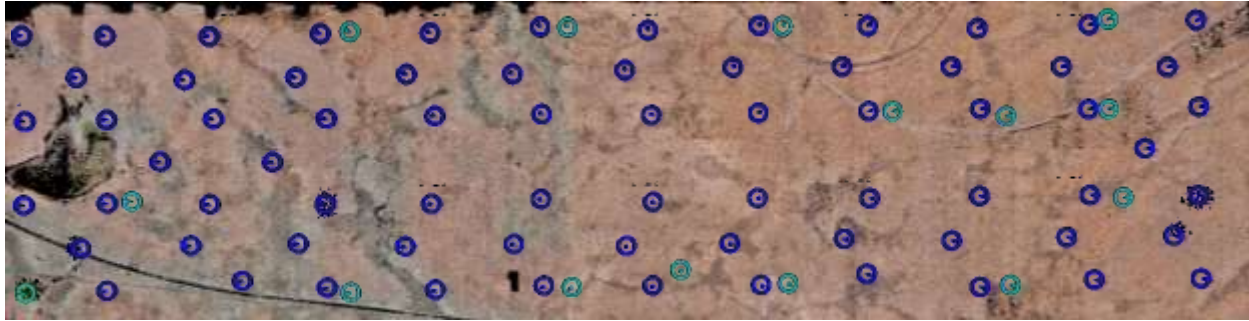
Figure 86. Location of 15 check points (CPs) shown as light blue markers vs. ground control points (GCPs) shown as dark blue markers.
