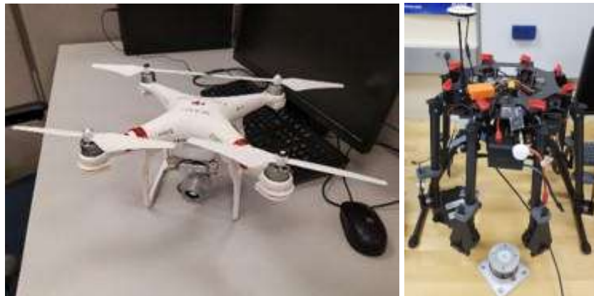
Figure 13. FIU's photogrammetry (left) and LiDAR (right) mobile mapping systems.
