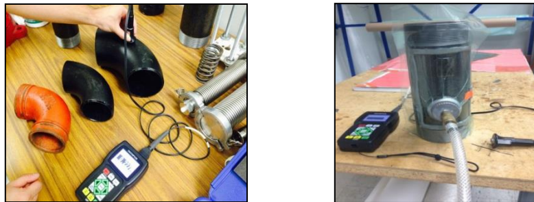
Figure 123. (a) Measurements using the Olympus UT system and (b) Vacuum tests.
