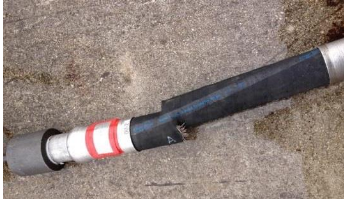
Figure 138. Ruptured HIHTL test specimen.
