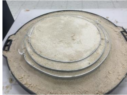
Figure 54. Test object with circles of sand of varying heights and diameters measured to mm resolution.
