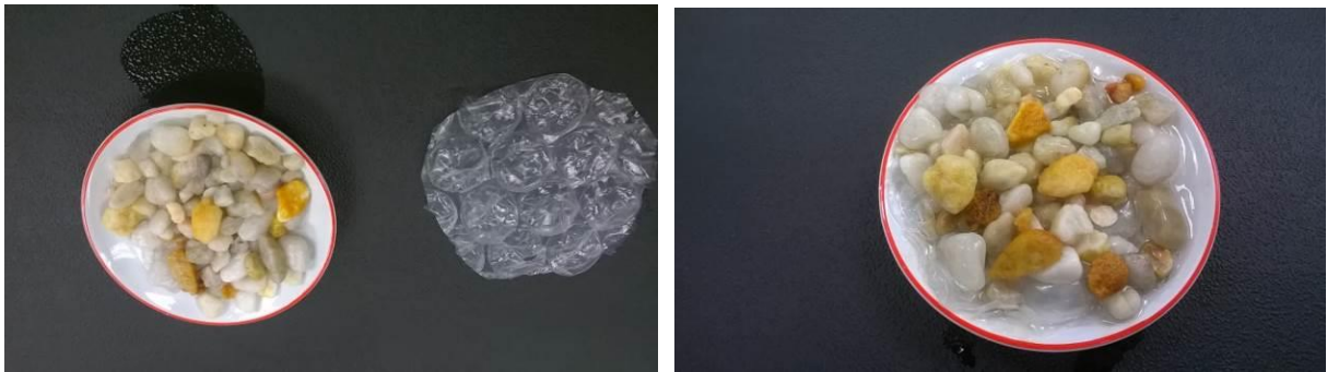
Figure 41. Plate of pebbles for sonar imaging and bubble wrap (left) and bubble wrap inserted under pebbles (right).
