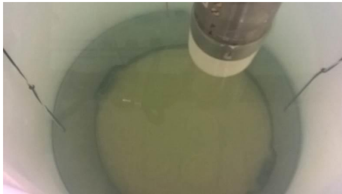
Figure 45. Photograph of plastic lid filled with sand on an aluminum plate on the tank bottom. The 3D sonar can be seen in the center top of the photograph.
