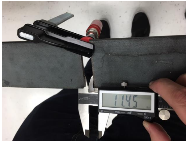
Figure 76. Test set up for navigation over a gap.
