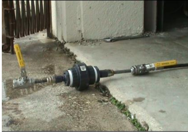
Figure 139. O-ring pressure test rig.
