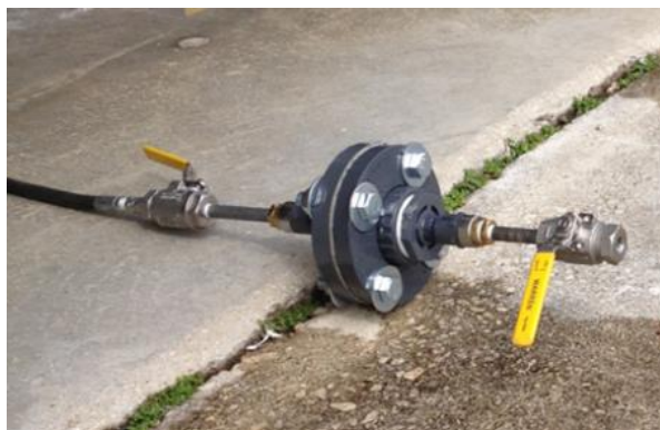
Figure 140. Gasket baseline pressure test rig.
