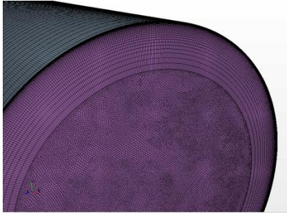
Figure 8. Computational grid containing 8.6m grid cells.
