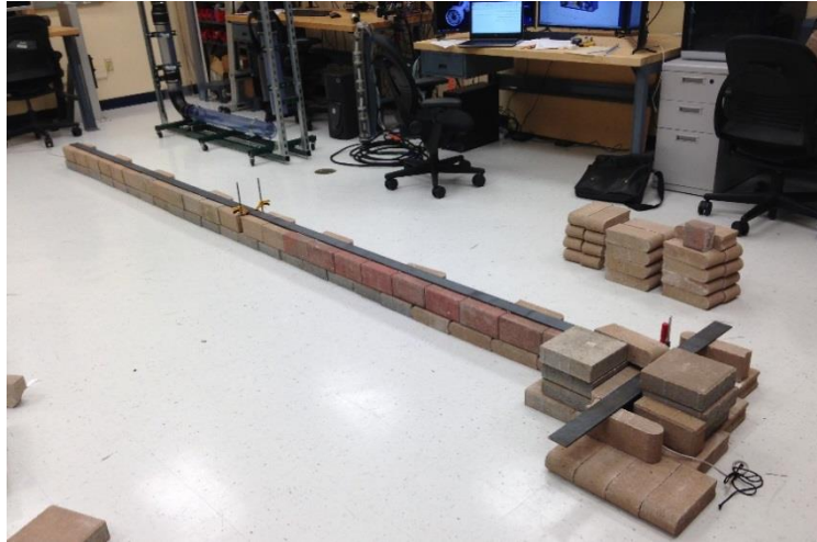
Figure 77. Laboratory scale test bed created for determining the pull force created by tether.
