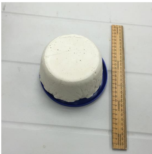
Figure 56. Plaster object used to test and correct volume calculation.
