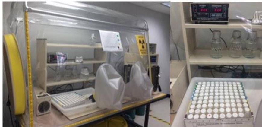
Figure 31. Sacrificial vials inside the anaerobic glove box filled with nitrogen gas, prepared to conduct the autunite biodissolution experiment.
