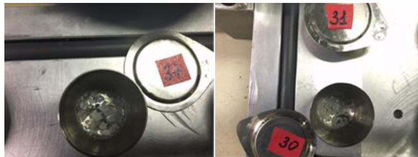
Figure 18. Condensation of water vapor forming a saturated solution on the bottom of crucibles.
