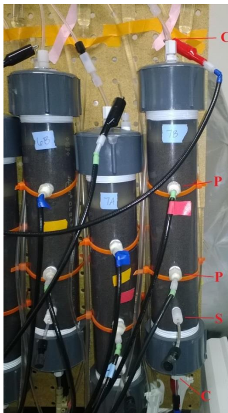
Figure 68. Structure of each column. C = Current Electrodes, P = Potential Electrodes, S = Microbe Injection Port.
