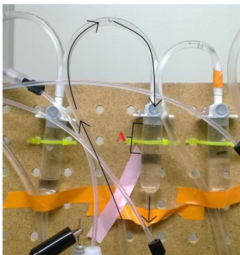
Figure 70. Air chambers used to prevent microbes swimming into influent; lines show flow of water through tubing. (A) Marks the pocket of air that prevents microbe migration.
