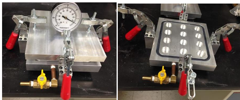
Figure 2. Isopiestic chambers for the solubility experiments fabricated in ARC’s machine shop.
