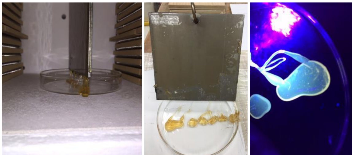
Figure 6. Sheet metal coupon placed in muffle furnace (left), fixative flowed from metal coupon into petri dish with exposure to heat at 250° F (middle); GloGerm transported from coupon to petri dish fluorescing under black light.
