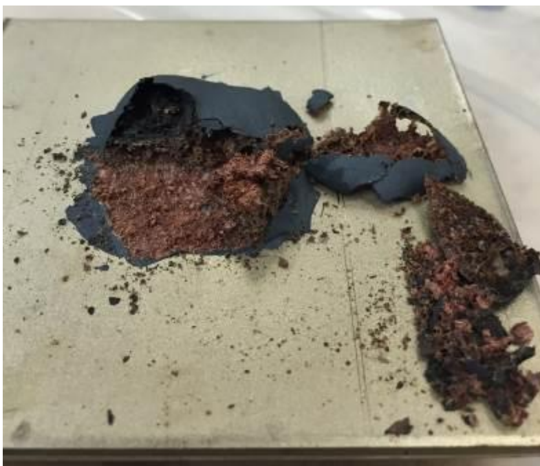
Figure 17. Fire Dam intumescent coating after exposure to 800° F.
