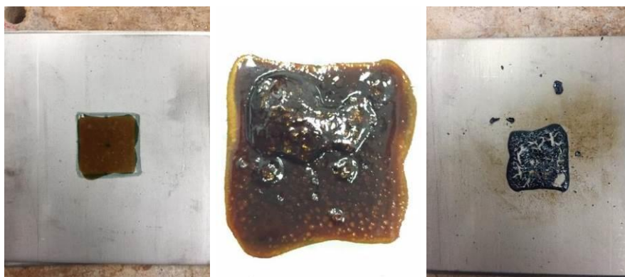
Figure 9. From left: Fixative A after exposure to 400°F, 600°F, and 800°F.
