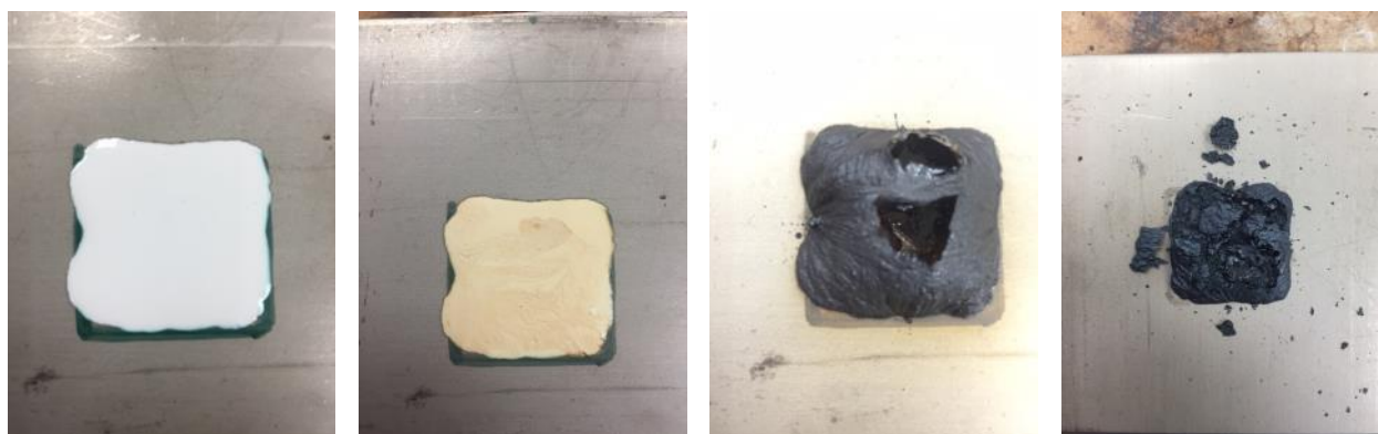
Figure 13. From left: Fixative E before exposure and after exposure to 500°F, 700°F, and 800°F.
