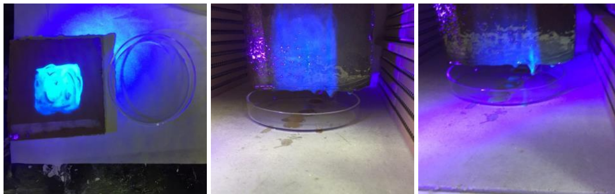
Figure 7. Red oak coupon and clean petri dish (left), fixative began to flow from coupon into petri dish with exposure to heat at 250° F (middle and right).
