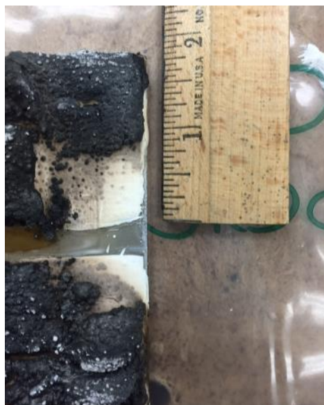
Figure 14. Charred intumescent coating provided thermal protection to bordering fixative.
