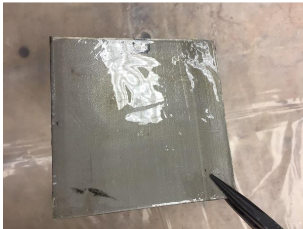
Figure 21. Back of stainless steel test coupon with Fixative A coating after front side (with FIREX IC) was exposed to direct flame.
