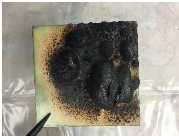
Figure 20. Stainless steel test coupon with FIREX intumescent coating after exposure to direct flame.
