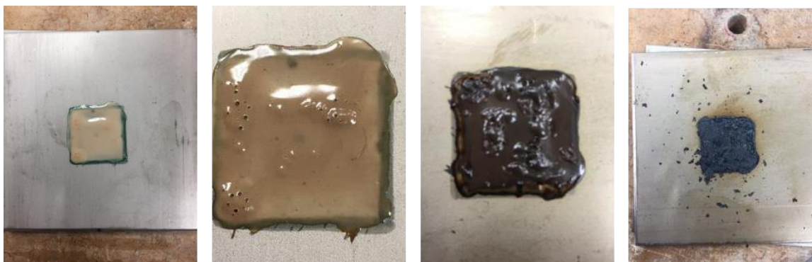
Figure 10. From left: Fixative B after exposure to 200°F, 400°F, 600°F, and 800°F.
