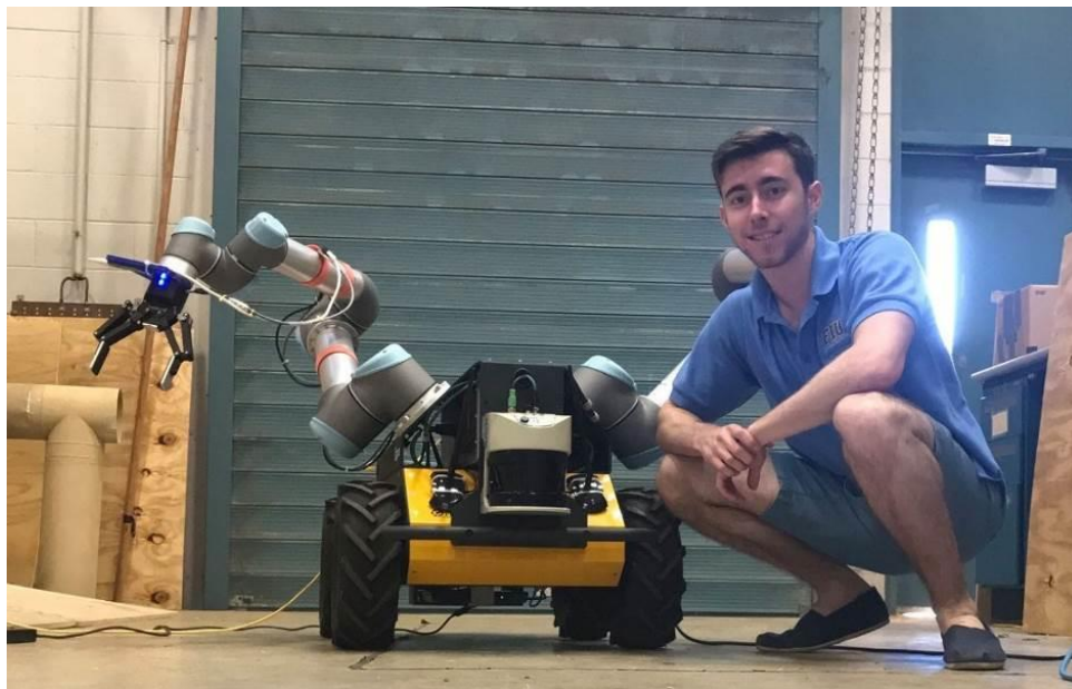
Figure 3. DOE Fellow Michael DiBono pictured with the robotic system developed for inspection and radiation surveying of CAEX.
