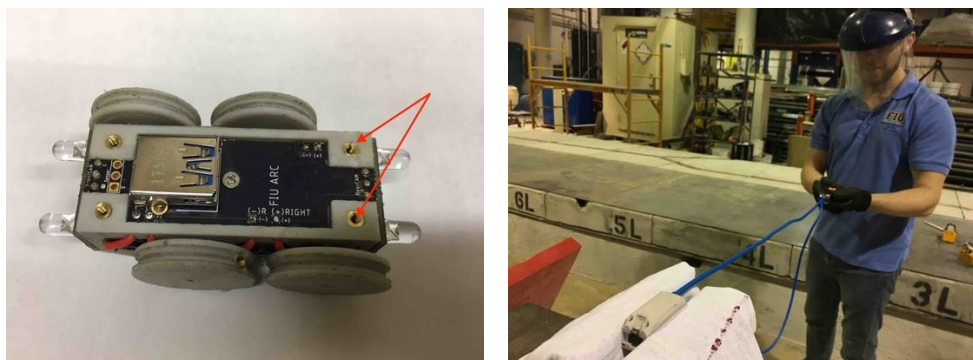
Figure 36. Screw holders at red arrows (left) for securing the hoop and the connectors to the inspection tool and performing a pull test for tether strength (right).
