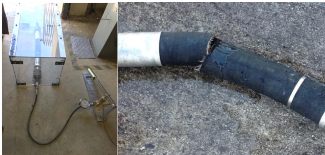
Figure 96. Hose rupture test apparatus (left) and ruptured hose section (right).
