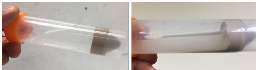
Figure 15. Test of cohesiveness of a fully settled kaolin bed in water.
