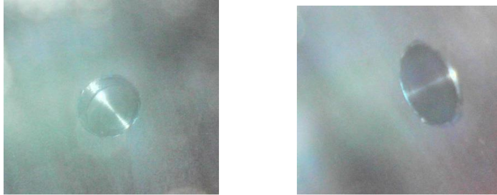
Figure 85. Endoscope image of the pipe with original coupon (left) and machined coupon (right).
