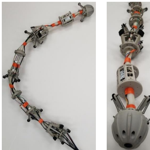
Figure 52. Crawler with sensor module.
