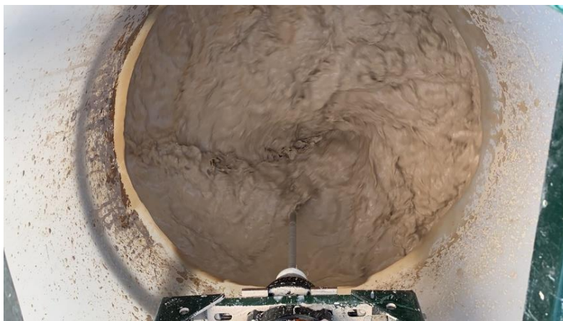
Figure 16. Performance testing of the mixer with 60 gallons of material in the tank.
