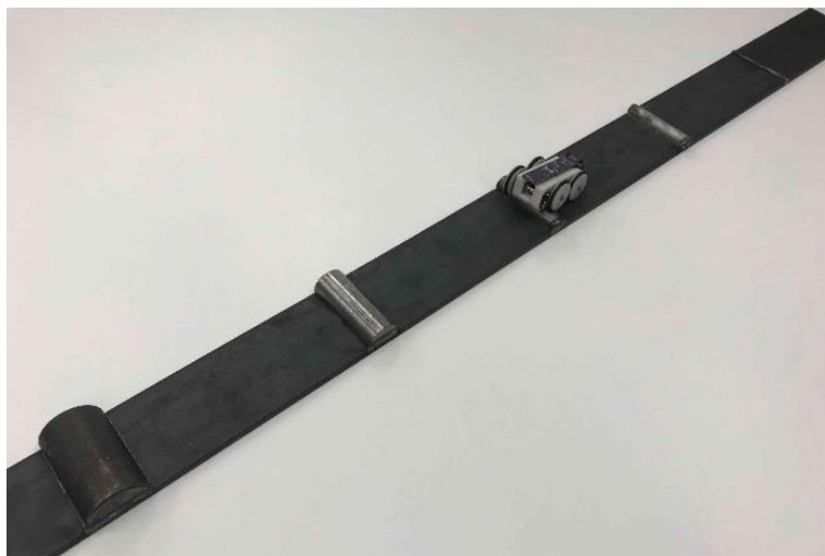
Figure 32. Weld seams of increasing height from 0.1 to 0.75 inches.
