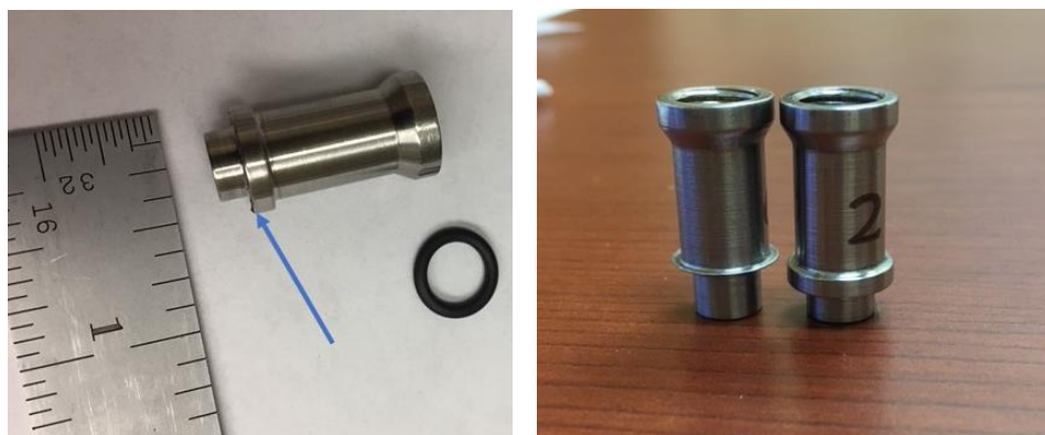
Figure 84. Coupon surface to be milled (left) and coupons before and after machining (right).
