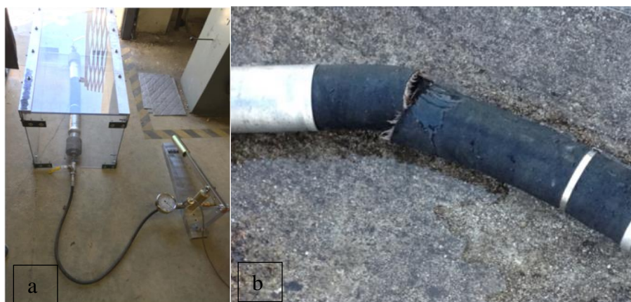
Figure. 94. Hose burst testing: burst pressure test apparatus (left) and ruptured hose section (right).
