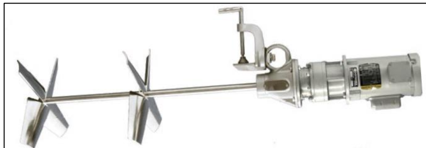
Figure 83. Sand water mixer [5].
