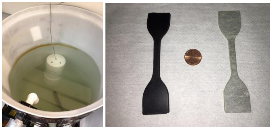
Figure 90. Coupon aging vessel (left) and EPDM & Garlock® coupons (right).
