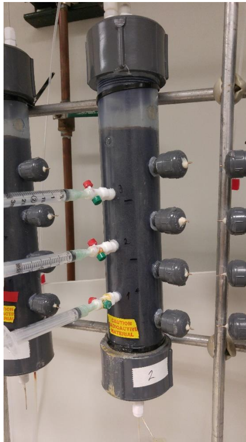
Figure 5 Image of column showing settling of sediment at the top.
