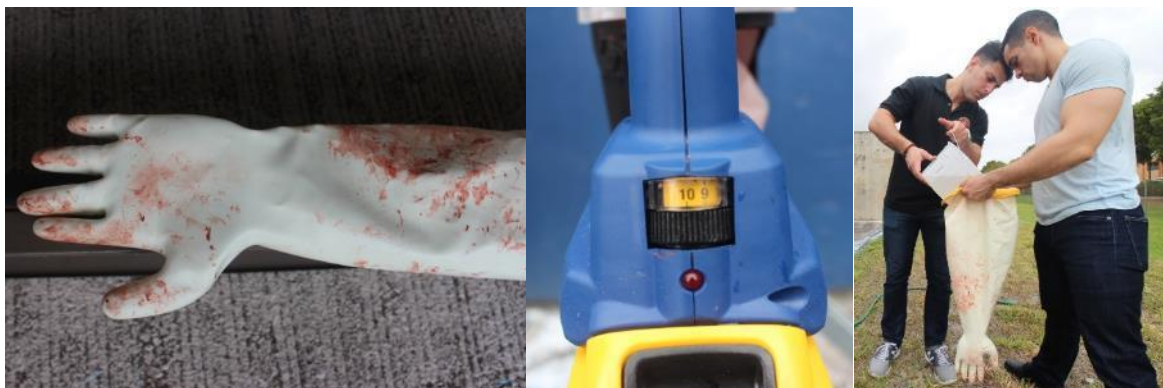
Figure 10. Testing impact of direct spraying on glovebox gloves: glove (left), sprayer setting (middle), and leak testing (right).
