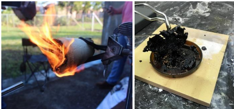
Figure 20. Initial testing of selected foam products: direct flame (left) and muffle furnace (right).
