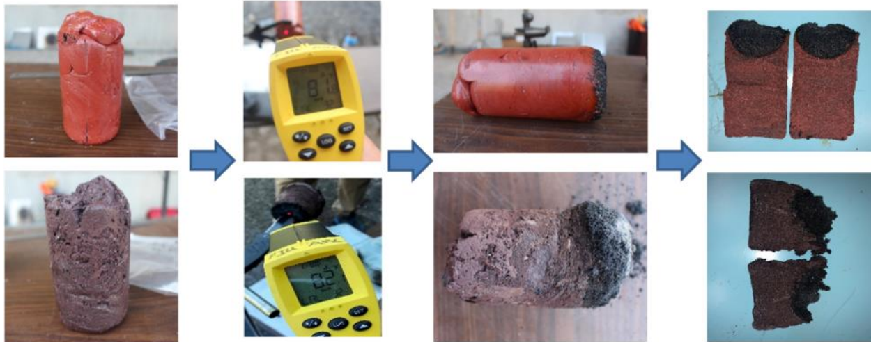
Figure 23. Intumescent foam testing.
