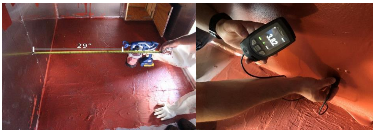
Figure 9. Testing sprayer at increased standoff distance.
