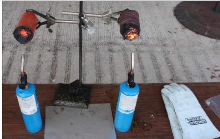
Figure 21. Experimental setup for direct flame testing.
