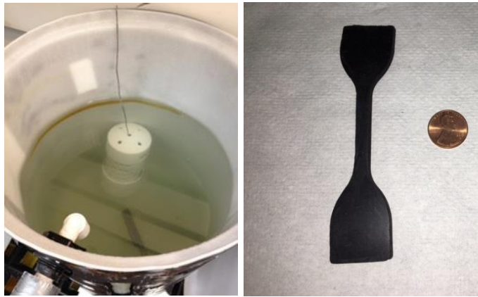
Figure 71. Coupon aging vessel (left) and EPDM dog bone (right).
