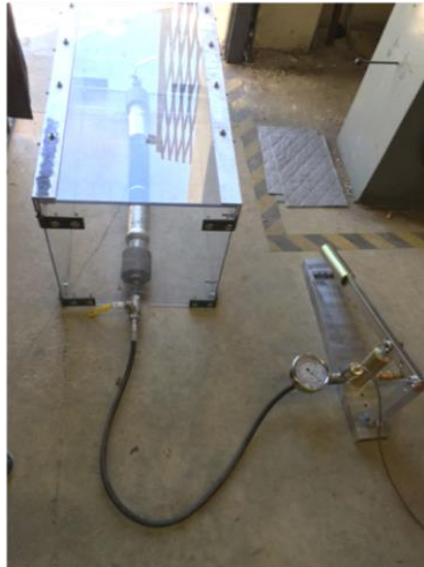
Figure 74. Hose burst test apparatus.
