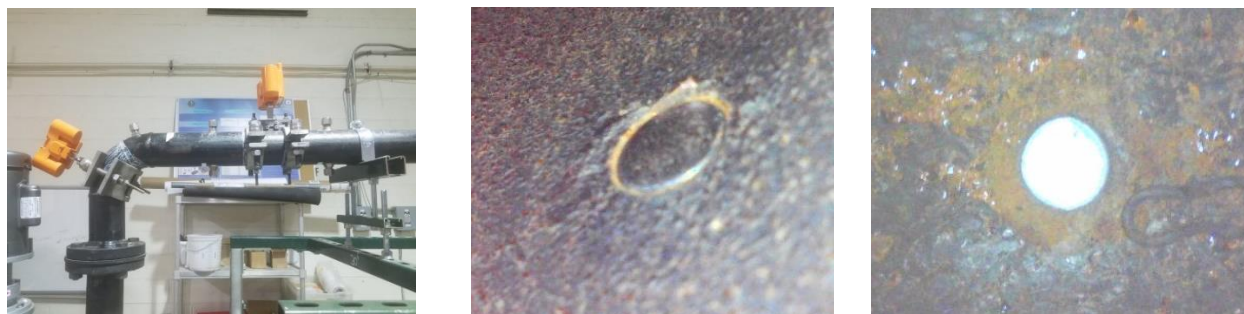
Figure 54. SRNL Coupons on the pipe loop, endoscopic images of the pipe internal surface with the coupons.
