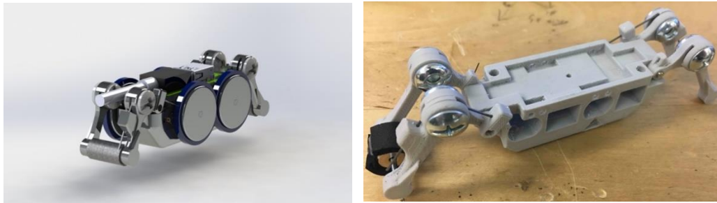
Figure 10. (Left) CAD drawing of the back view of the modified rover with magnetic arms. (Right) Initial 3D printed prototype to evaluate the feasibility of the modified design.
