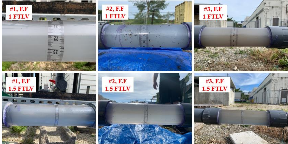
Figure 5. Pipeline condition after flushing with 1 (up) and 1.5 (bottom) line volume of water from fully-flooded (F.F) initial conditions; sections #1, 2, and 3 are start, middle, and end of loop, respectively.
