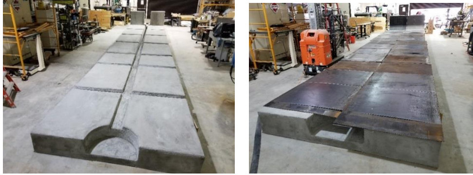
Figure 45. The full-scale mockup foundation.
