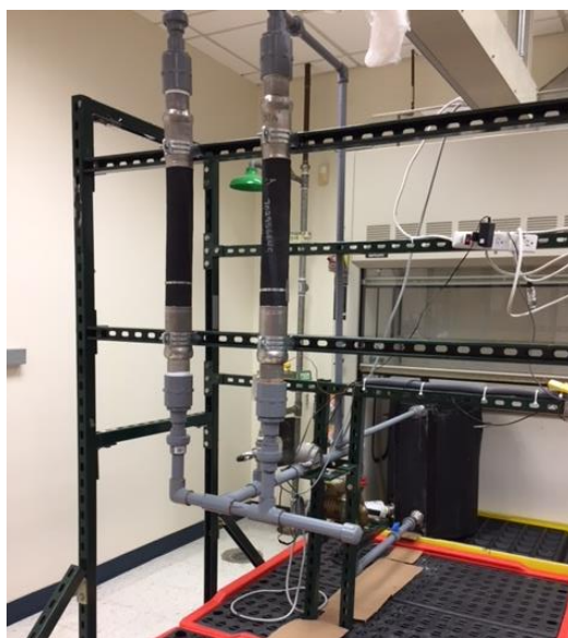
Figure 69. Water only aging loop.
