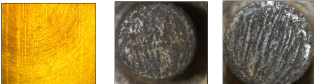
Figure 61. a) New coupon surface; b) Coupon 1 (after testing); c) Coupon 2 (after testing).
