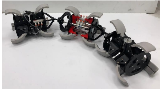
Figure 36. Mother pipe crawler prototype.
