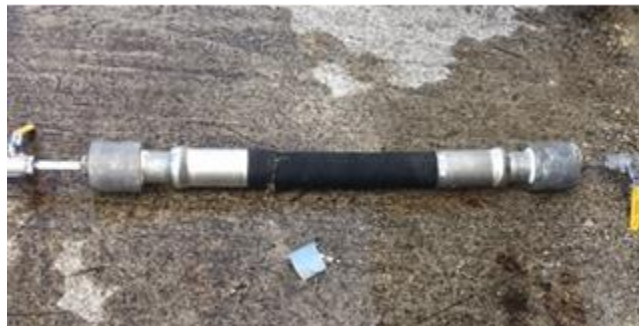
Figure 76. Ruptured HIHTL specimens WO-02.
