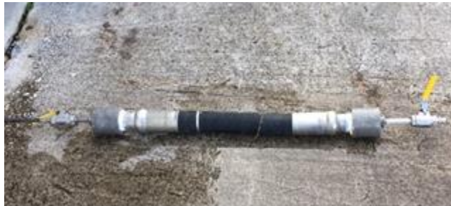
Figure 75. Ruptured HIHTL specimen WO-01.
