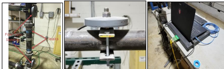
Figure 56. a) Fiber optic sensors on the loop; b) single transducer (LCM-500); c) LCM-2500 Interrogator and user control station.
