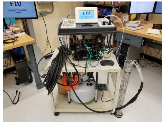
Figure 37. Pneumatic crawlers control box.
