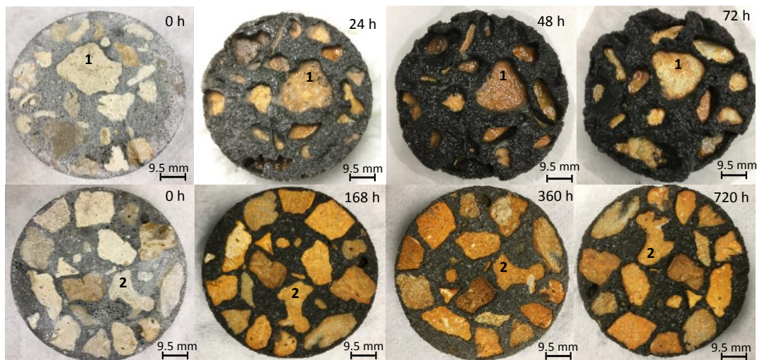
Figure 48. Images of concrete specimens (sample 2) immersed in 0.025M (top) and 0.5 M (bottom) nitric acid solutions. (The numbers 1 and 2 identify the same coarse aggregate for the two tested specimens at different times. Samples were wet when the pictures were taken, except for the control sample).
