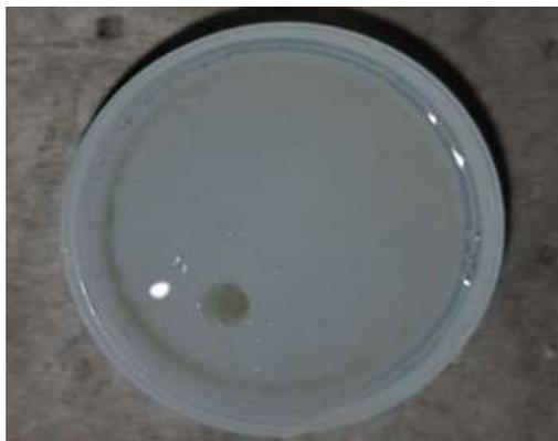
**Figure 22. Suspension of white solid observed inside reactor from SPFT experiment at 70°C. The circle in the bottom left indicates where the suspension has held shape from the presence of the tubing.**
