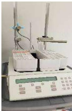
**Figure 17. Spectrum IS-95 interval collector for SPFT experiments.**
