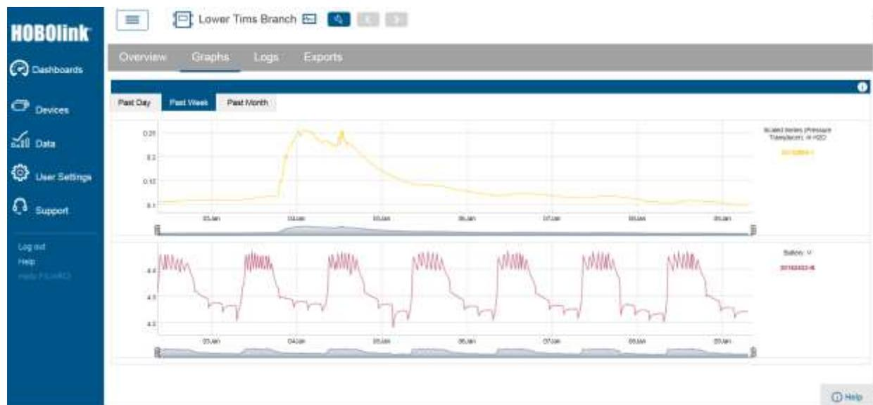
**Figure 55. Screenshot of the graphed water level data and battery performance for the Lower Tims Branch HOBO data logger for a 1-week time period viewed through the HOBOLink website. Graphs can be generated for recorded data on a daily, weekly or monthly basis.**
