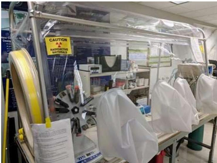
**Figure 7. Anaerobic glovebox with 98%  $\text{N}_2$ : 2%  $\text{H}_2$  atmosphere where pertechnetate reduction experiments are currently taking place.**
