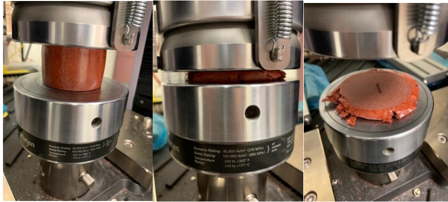
Figure 21. Compression process for I-H cylindrical sample.
