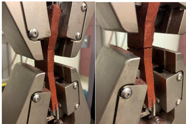
Figure 19. Foam sample before failure (left) and after failure (right).
