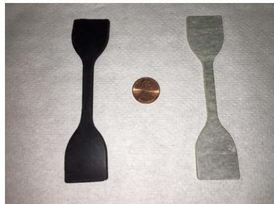
Material Properties Test Coupons: EPDM (left) and Garlock® (right)
