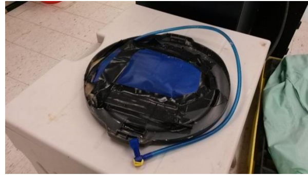
Fig. 3. Air bladder with metal weights underneath taped to a plastic lid.
