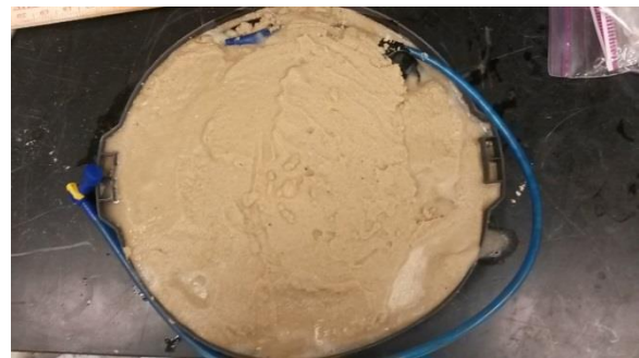
Fig. 4. Same air bladder covered with paver sand to create object to be imaged by the 3D sonar.
