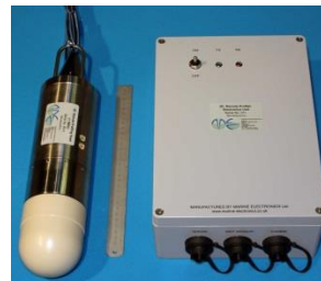
Fig. 1. 3D profiling sonar and controller
