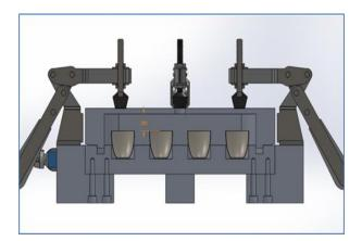
Diagram of isopiestic chamber assembly with aluminum block and nickel crucibles.
