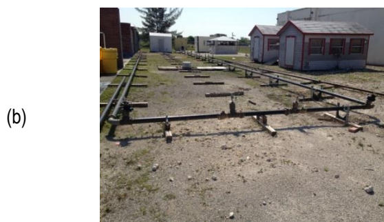
Asynchronous Pulsing Method: (a) Principles of Operation (b) Engineering-Scale Test Bed for Asynchronous Pulsing
