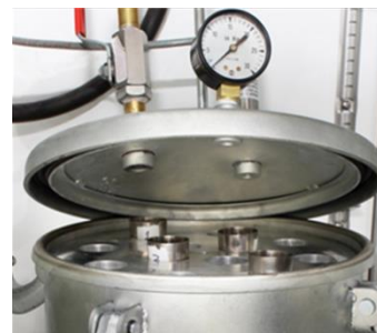
Isopiestic chamber to conduct solubility experiments; aluminum block with holes to hold nickel crucibles
