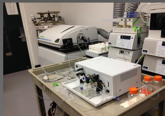
Coupling of a Flow Injection System (FIAS 400) to ICP-MS for analyzing mercury isotopes
