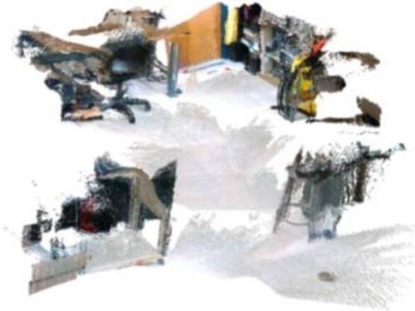
**Figure 90. Improved captured map by fused data from a 3D camera.**
