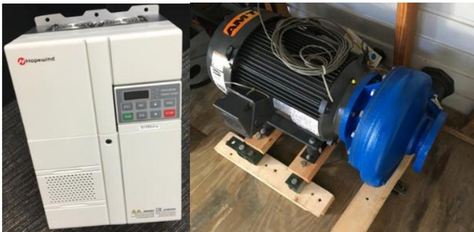
**Figure 4. (Left) HopeWind VFD; (Right) AMT 427B-95 15 HP Slurry Pump.**
