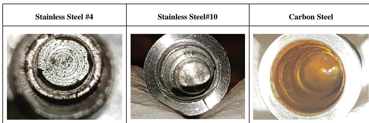
Figure 118. Visual corrosion inspection of the CS and SS coupons (2M).
