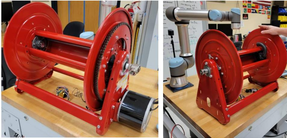
**Figure 59. Tether reel and potential slip-ring.**
