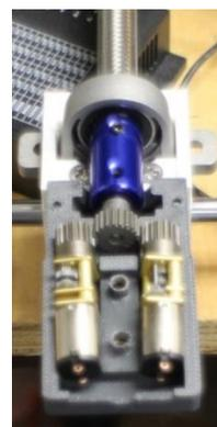
**Figure 81. New gear motor module.**
