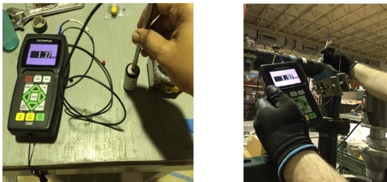
**Figure 110. a) UT sensor calibration and b) real-time coupon thickness measurement.**
