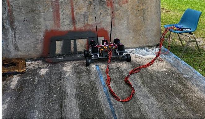
**Figure 69. Power delivery setup to multi-fan platform.**
