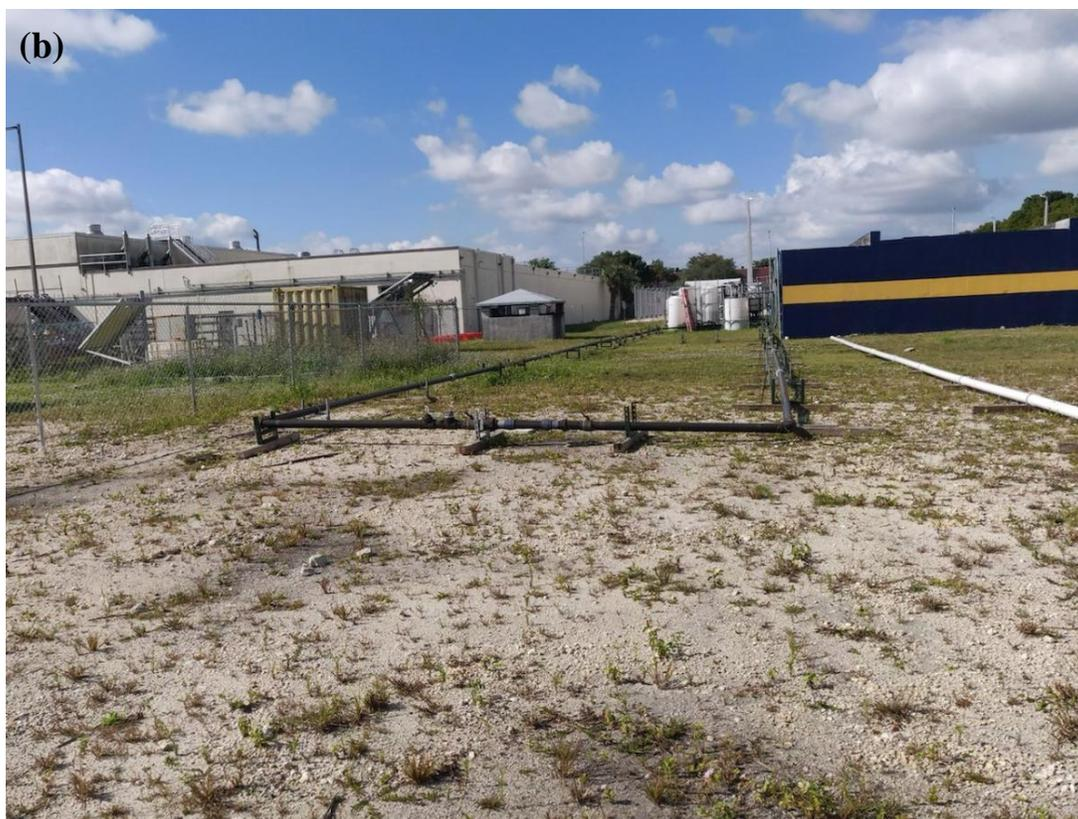
**Figure 3. (a) CAD Model of 330-foot flushing loop used for second round of testing; (b) Assembled 330-foot flushing loop.**
