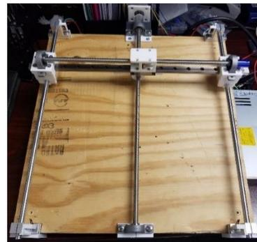
Figure 77. Partially assembled coating mechanism with portable power supply.
