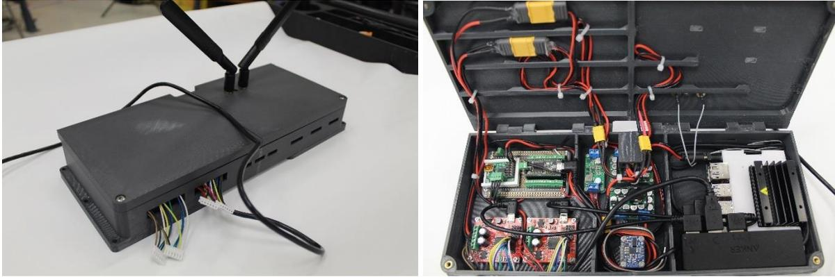
**Figure 67. Completed control system unit.**
