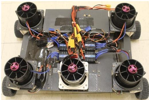
**Figure 65. Top view of multi-fan platform with control box unit.**
