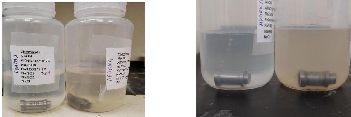
Figure 117. SRNL coupon immersion tests initial (Day 1) (left) and current (Day 35) (right).
