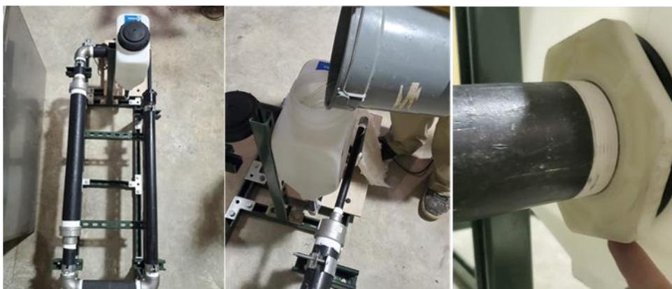
Figure 116. a) Bench scale loop, b) water testing and c) pipe leak.
