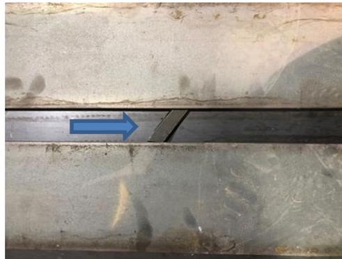
**Figure 17. Oblique/Blunt weld seam.**
