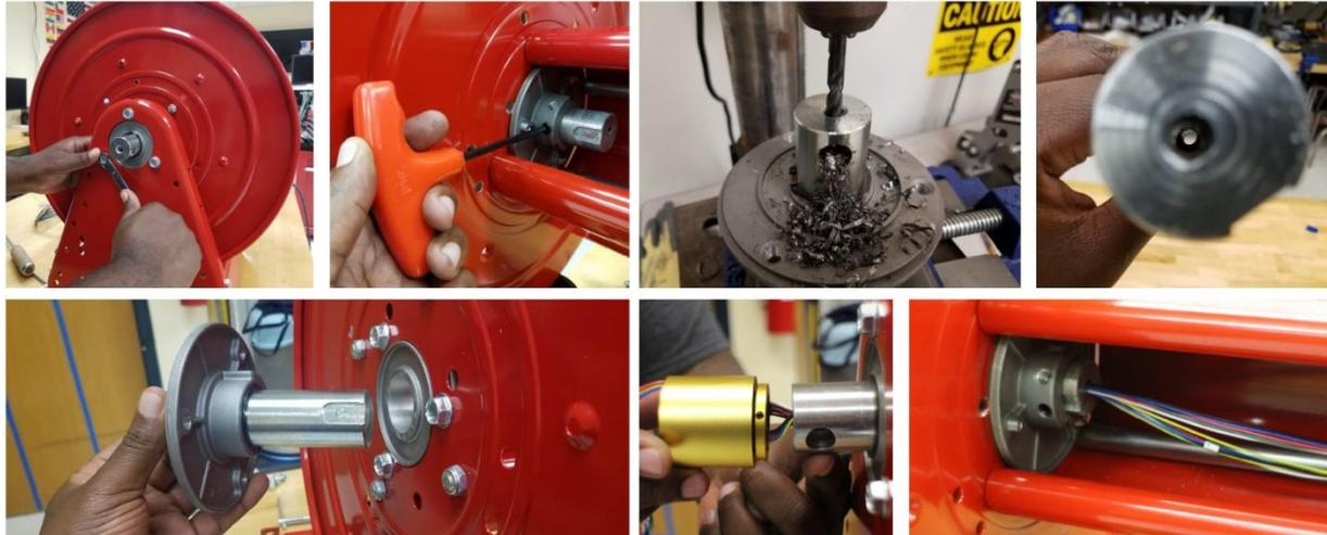
**Figure 60. Ethernet slip-ring integration.**
