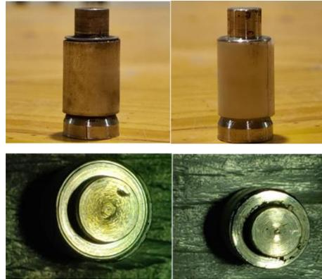
**Figure 111. Eroded Coupon surfaces removed from the elbow and bottom sections of the pipe.**
