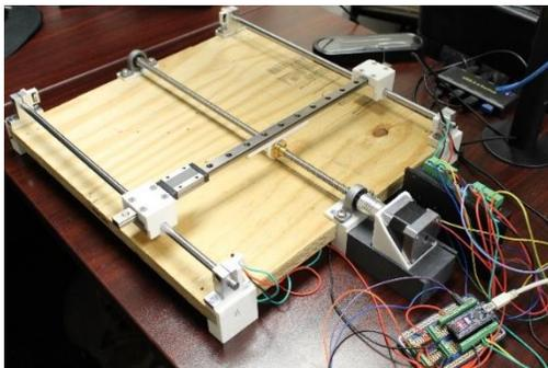
Figure 76. Lead screw-based coating application system.
