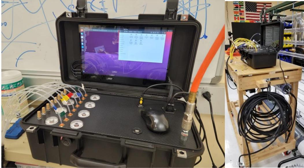
**Figure 58. Pipe crawler portable control box.**
