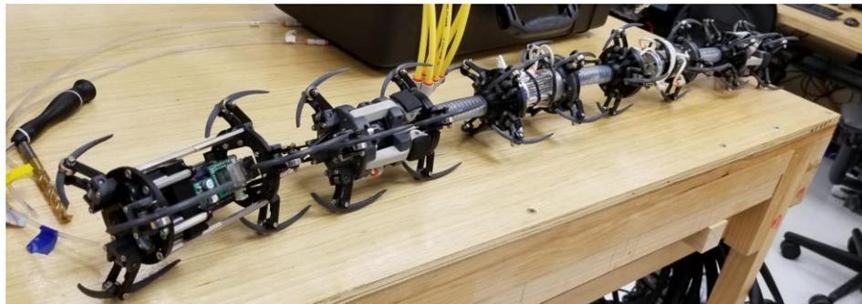
**Figure 54. Current pipe crawler prototype.**
