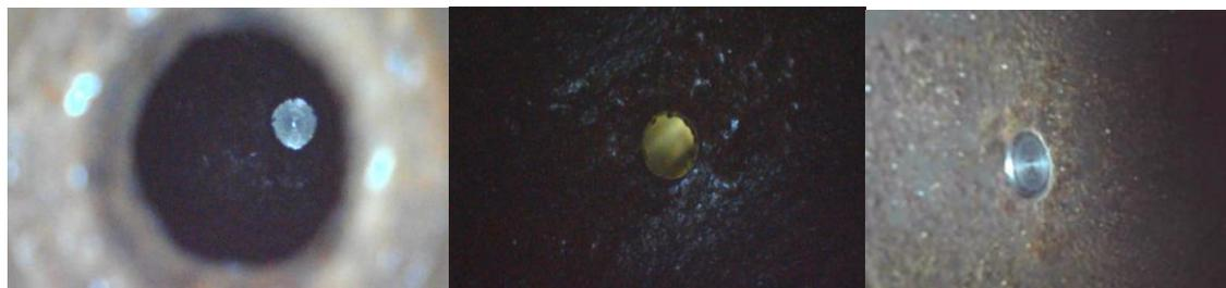
**Figure 109. Borecope images of the coupons in the pipe loop.**
