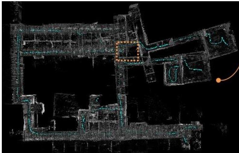
**Figure 97. Closed loop failure in the localization algorithm.**
