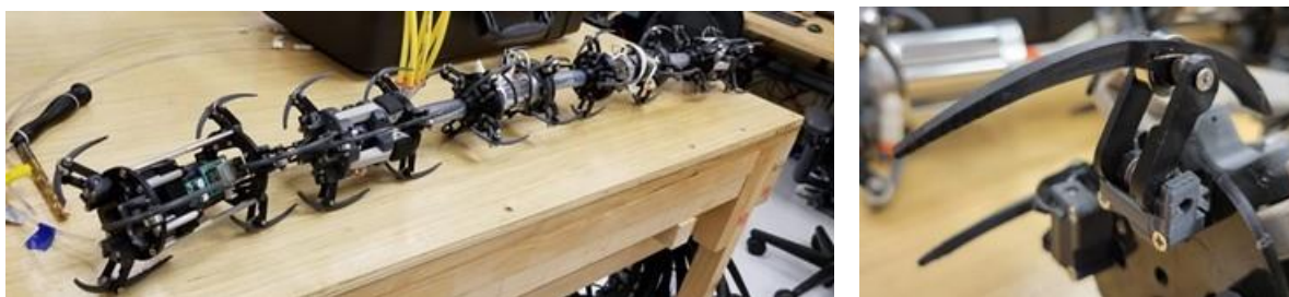
Figure 23. Current pipe crawler prototype (left) & improved guides (right).
