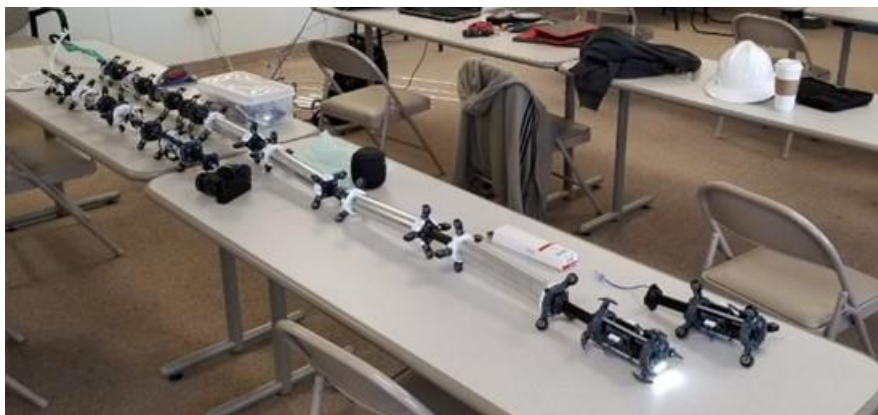
Figure 53. Initially designed gripper module (left) and modified rubber strips (right).
