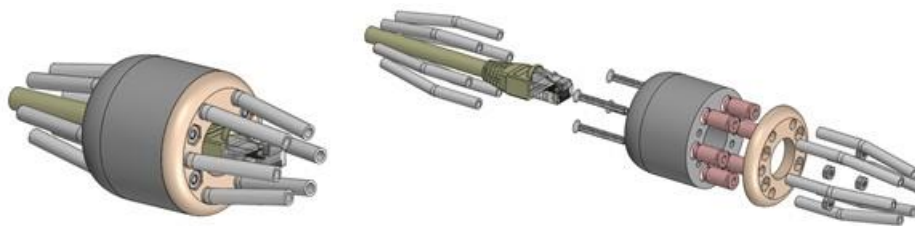
Figure 35. Tether “egg” for quick detachment.
