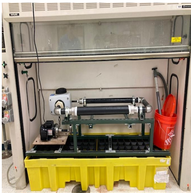
Figure 102. Assembled bench scale loop inside the fume-hood for caustic simulant testing.
