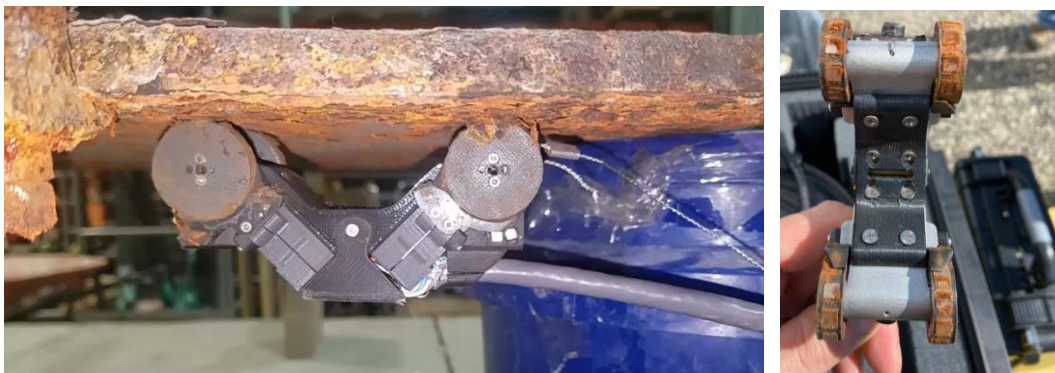
Figure 15. FIU’s in-house testing (left) and retriever rover after AP-105 DST deployment (right).
