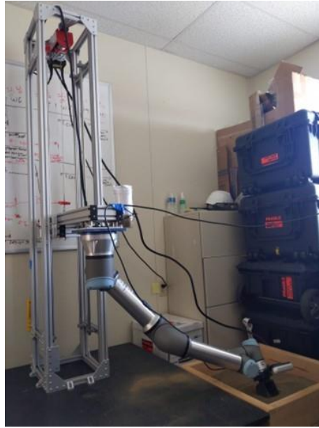
Figure 87. UR5e off-riser sampling demonstration scooping simulant.
