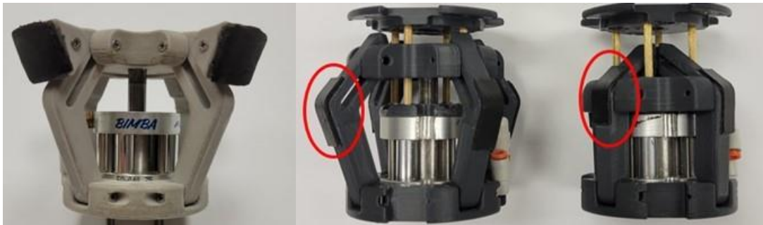
Figure 25. Original (left) and redesigned gripper arms (center and left).
