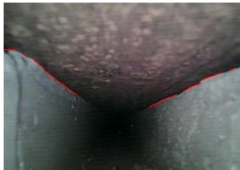
Figure 20. Channel edge detection on FIU’s full-scale mockup channel.
