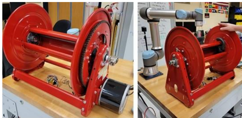
Figure 38. Motorized cable reel.
