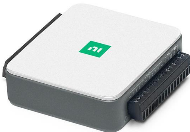
Figure 6. NI-USB6001 Multifunction I/O data acquisition unit.
