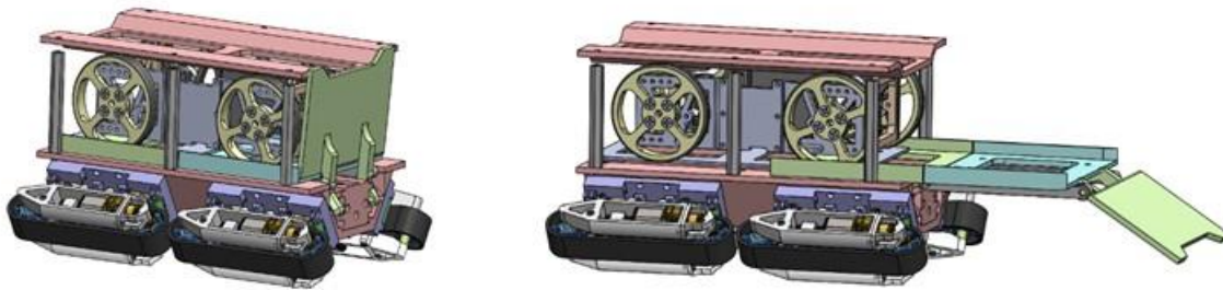
Figure 56. Model of rover in housing module with deployable ramp.
