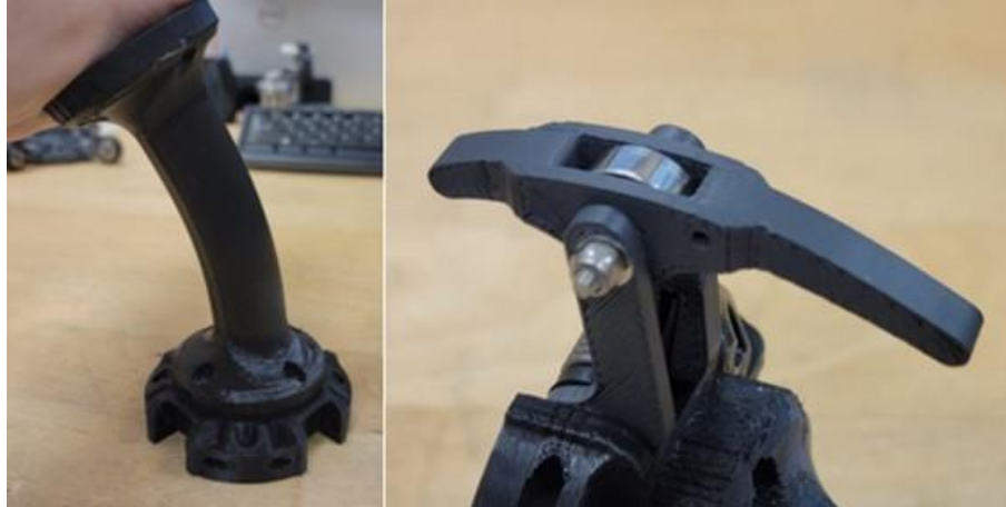
Figure 24. 3D printed inter-module flexible connection (left) and strengthened guides (right).
