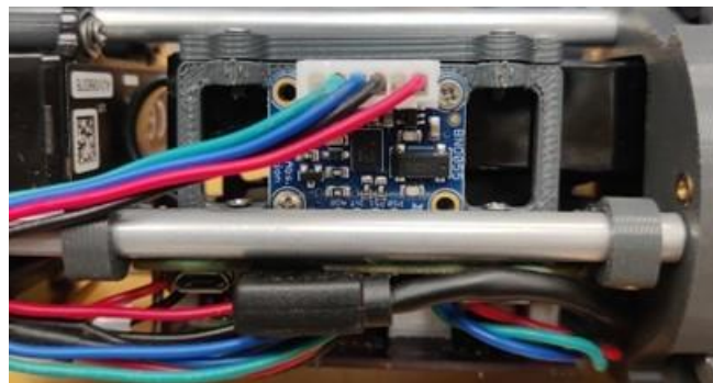
Figure 44 . BN055 IMU in front module.
