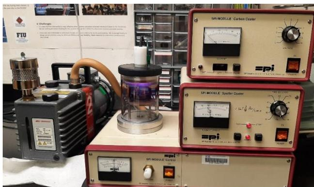
**Figure 9. Instrument used to gold coat samples.**
