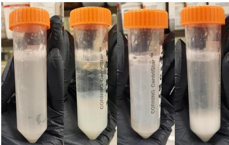
**Figure 2. Precipitate formed in week 6 for Scenarios A, B, C, and D (left to right).**
