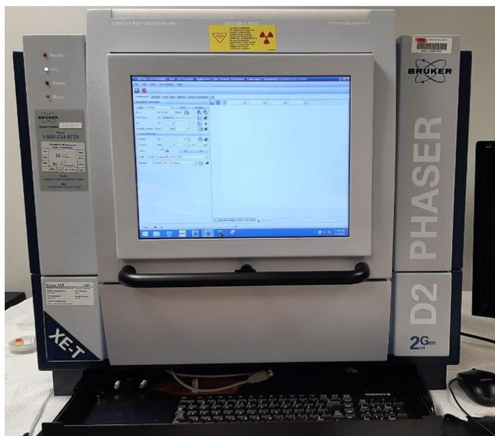
Figure 6. Bruker D2 PHASER XRD instrument.
