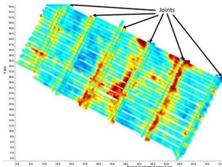
**Figure 35. Depth Slice of the Surveyed Path (Image from Sensors & Software Inc.).**
