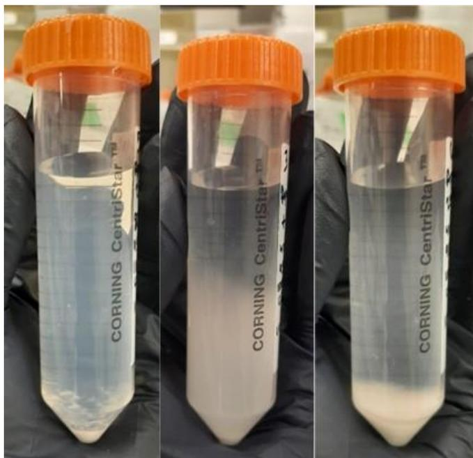
**Figure 3. Amorphous precipitate formed in week 1 for Scenarios A, C, and D (left to right) with uranium.**
