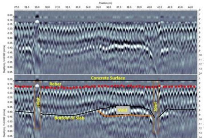
Figure 34. Raw Data of the Interpreted Voids (Image from Sensors & Software Inc.).
