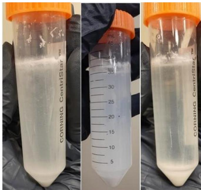
Figure 4. Crystalline precipitate formed in week 5 for Scenarios A, C, and D (left to right) with uranium.
