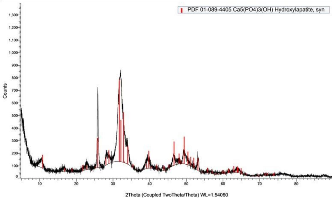
**Figure 28. Matched XRD pattern for Scenario D with uranium.**
