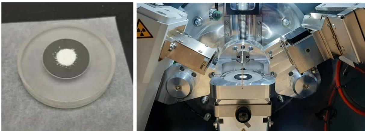
Figure 7. Hydroxyapatite powder on sample holder prepared for XRD analysis.
