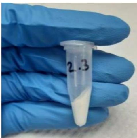
Figure 5. Dried HA precipitate formed during synthesis.
