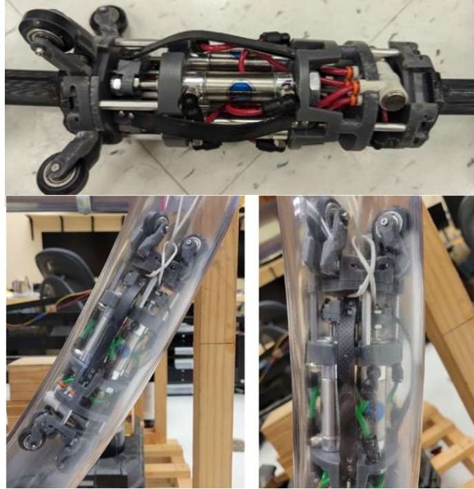
Figure 86. Improved gripper module with independent blades.
