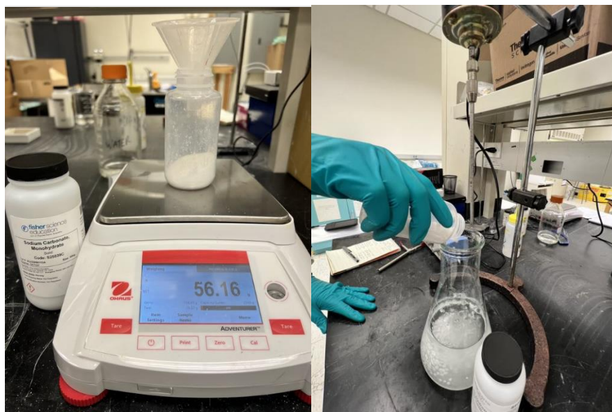
Figure 154. Simulant mass measurement (left) and experimental set up for mixing the salt simulants (right).
