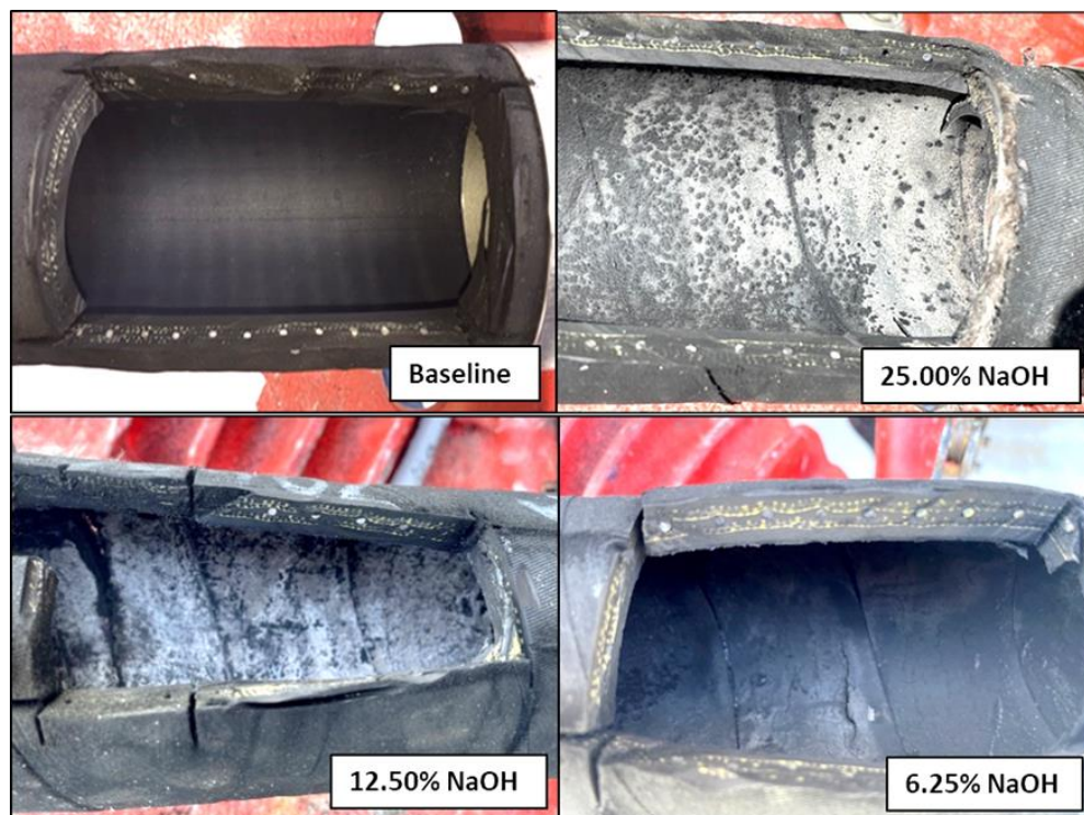
Figure 207. Comparison of the inside of unaged and aged HIHTL specimens.
