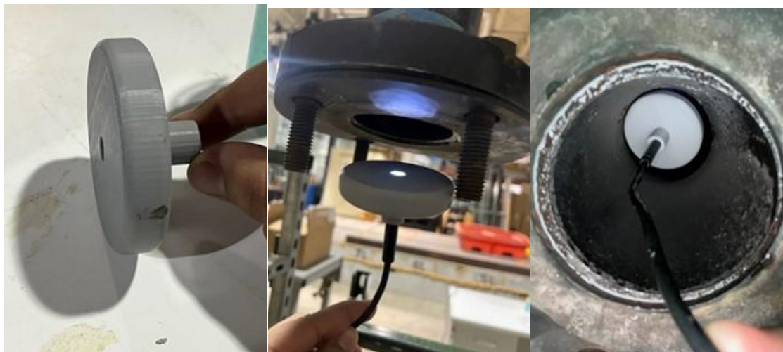
Figure 133. Pipe adapter - 3D printed part (left), fitted borescope (center) and in the pipe section (right).
