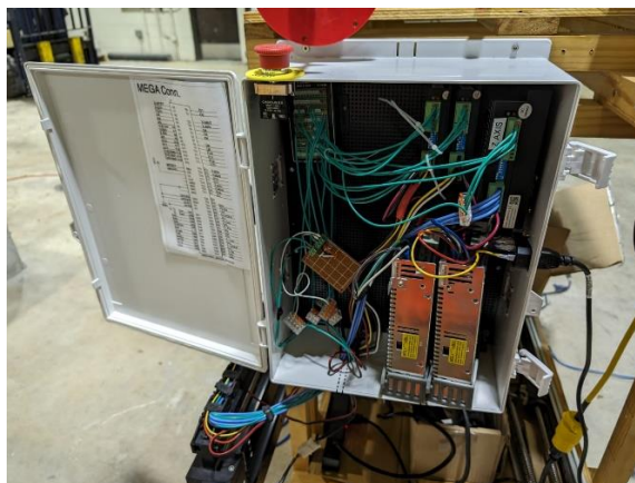
Figure 121. 3D printer's upgraded control panel.
