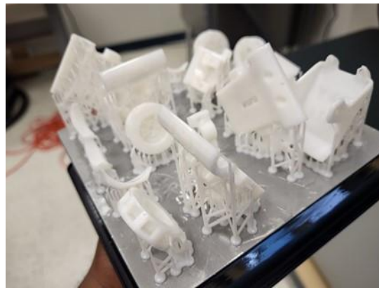
Figure 45. Miniature Rover resin parts before post-processing.
