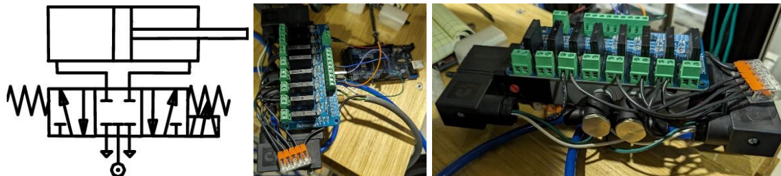
Figure 109. Pneumatic joint’s three-position control schematic (left) and prototype (right).
