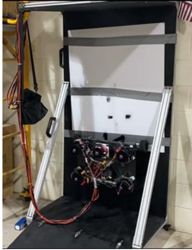
Figure 18. Deployment of spray material on vertical surface.
