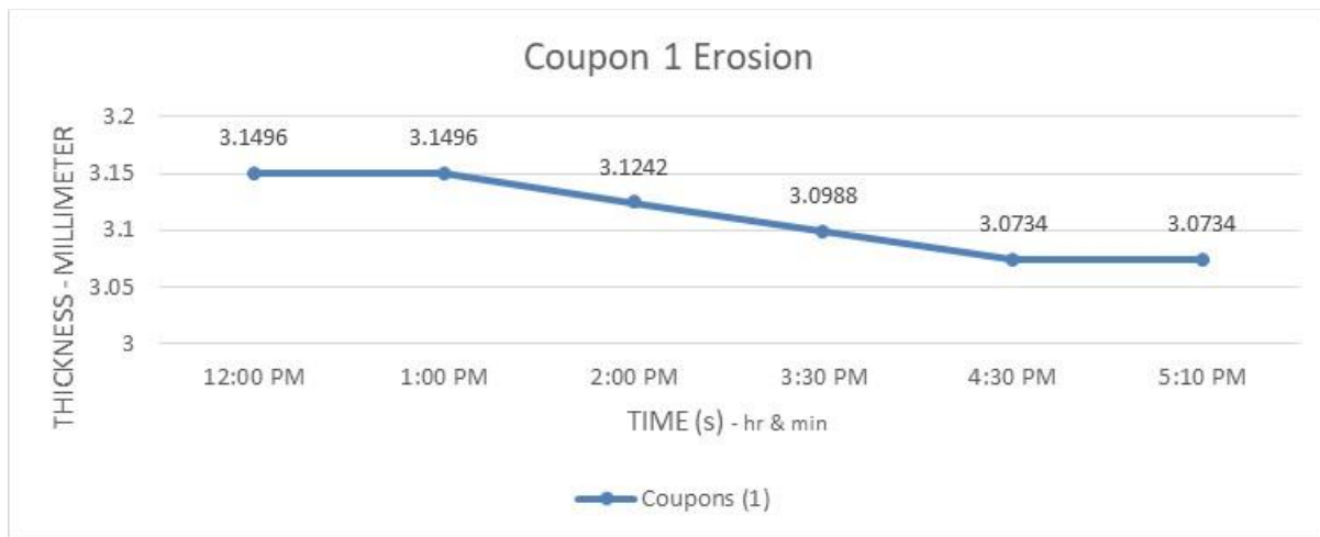
Figure 135. Degradation in coupon placed near the elbow.
