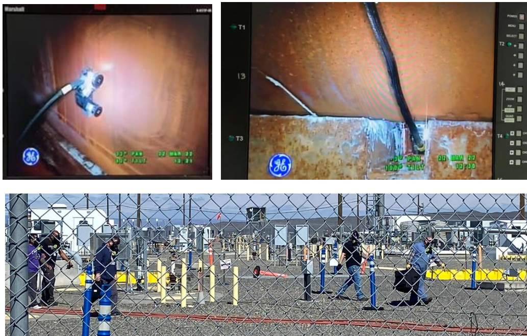
Figure 43. FIU's miniature inspection rover deployment at AP-105 DST.
