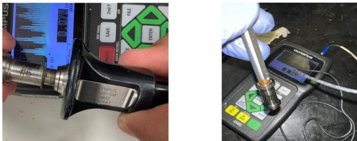
Figure 145. UT measurement of the coupon using two separate sensors (inner and outer coupon surface).
