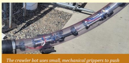
The crawler bot uses small, mechanical grippers to push and pull itself along the inside of a pipe.
