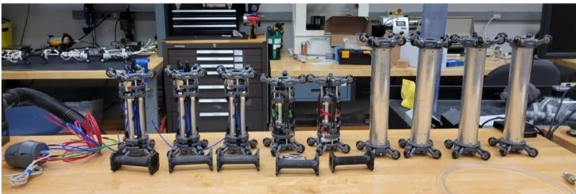
Figure 88. Pipe crawler improved modules.
