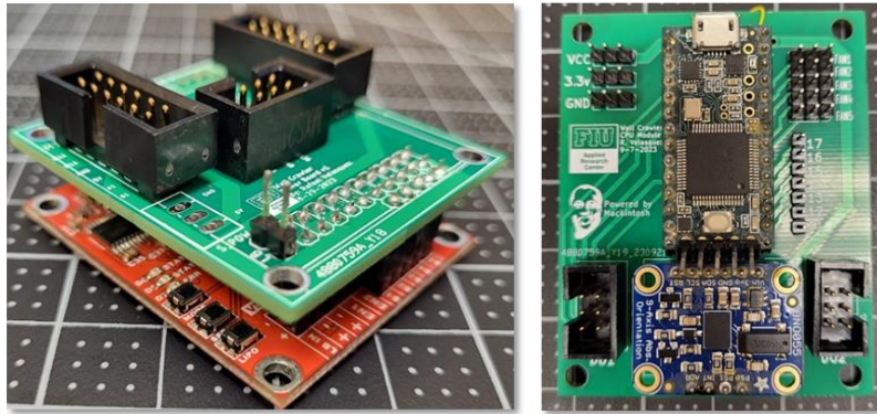
Figure 9. PCB modules for motor controller, microcontroller and IMU integration.
