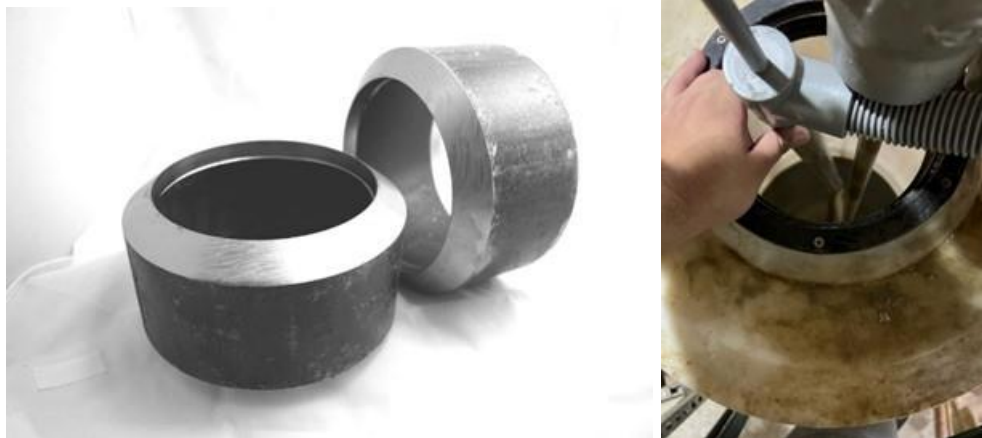
Figure 132. Pipe coupons (6-inch) for making the erosion coupons (left) and manual pump in the reservoir tank (right).
