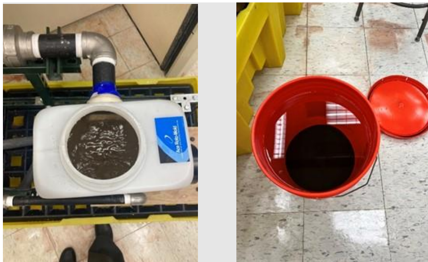
Figure 152. Caustic simulant solution in the tank (left) and after 3 weeks of settling (right).
