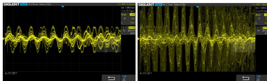
Figure 64. Grounded (left) and ungrounded (right) video feed.
