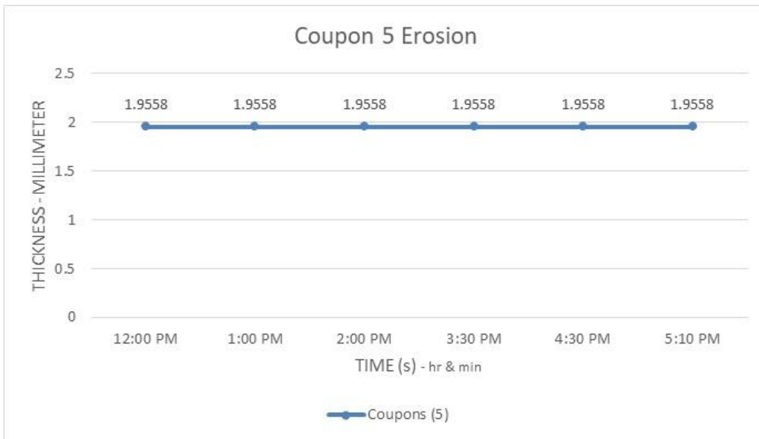
Figure 138. Degradation in coupon placed at the bottom of 3-inch section closer to the reducer.
