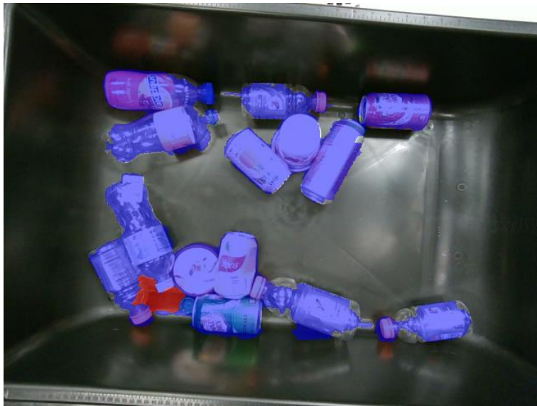
Figure 120. Example of the results from STEGO where blue pixels are convex polygons and red pixels are the holes within the convex polygons.
