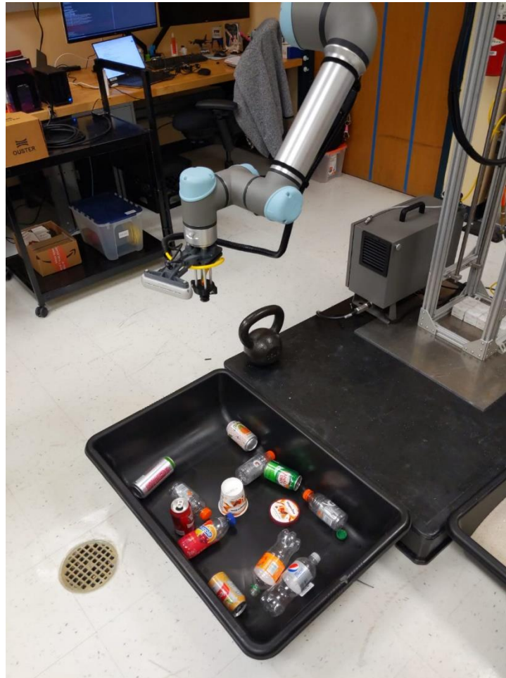
Figure 124. Image of the robotic arm which uses the computer vision models to determine what objects to collect and how to collect them (from their shape).
