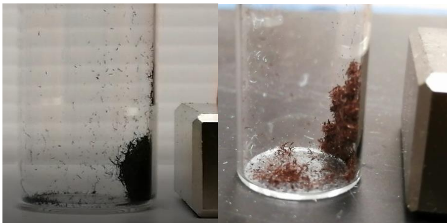
Figure 35. The magnetic field responsiveness of unheated mPDMS-MRs (left) and heated mPDMS-MRs (right).
