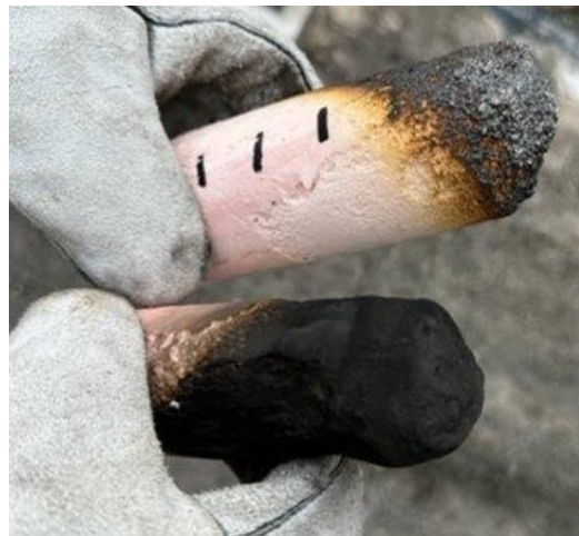
Figure 27. FoamBag™ flammability comparison with (top sample) and without (bottom sample) the Exolit AP-750 additive.
