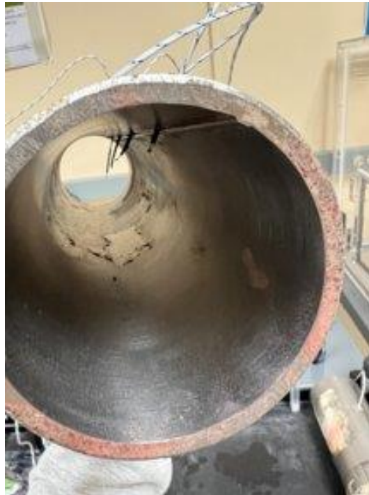
Figure 18. Pipe with thermocouples at varying depths.
