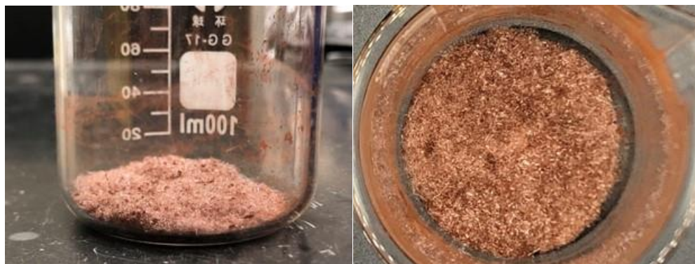
Figure 36. The mPDMS-MRs that were thermally oxidized at 370°C for 24h.
