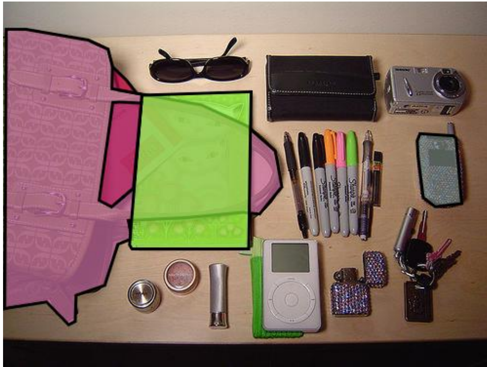
Figure 111. Example of an image in the COCO dataset and its corresponding pixel masks.
