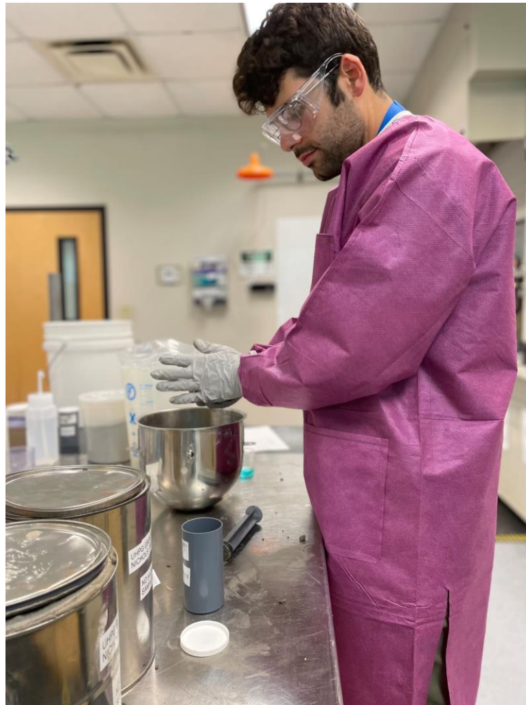
Figure 20. DOE Fellow, Gabriel Ceroni, mixing concrete mixtures for optimized 3D Printing Applications.
