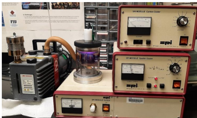
Figure 5. Instrument used to gold coat samples.
