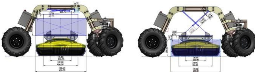
Figure 32. Robot's GPR antenna actuator.
