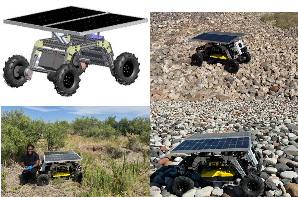
Figure 51. GPR mobile robot CAD design (top-left), GPR robotic platform Mexican Hat, UT deployment (top-right), GPR robotic platform deployment in Basin 6 west of the WIPP, New Mexico (bottom-left), and Rifle Colorado GPR robotic platform near the depression areas (bottom-right).
