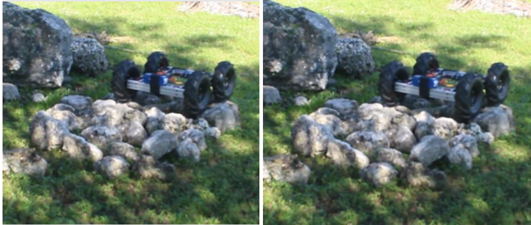
Figure 25. Preliminary rocky terrain traversal tests using an all-terrain wheeled robot.
