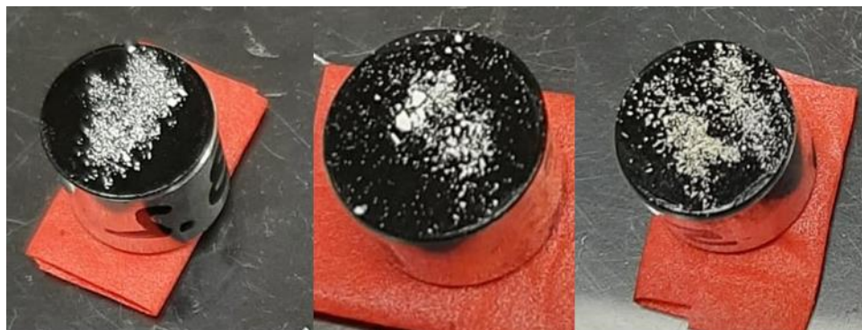
Figure 4. Dried HA Precipitate Prepared for SEM Analysis.
