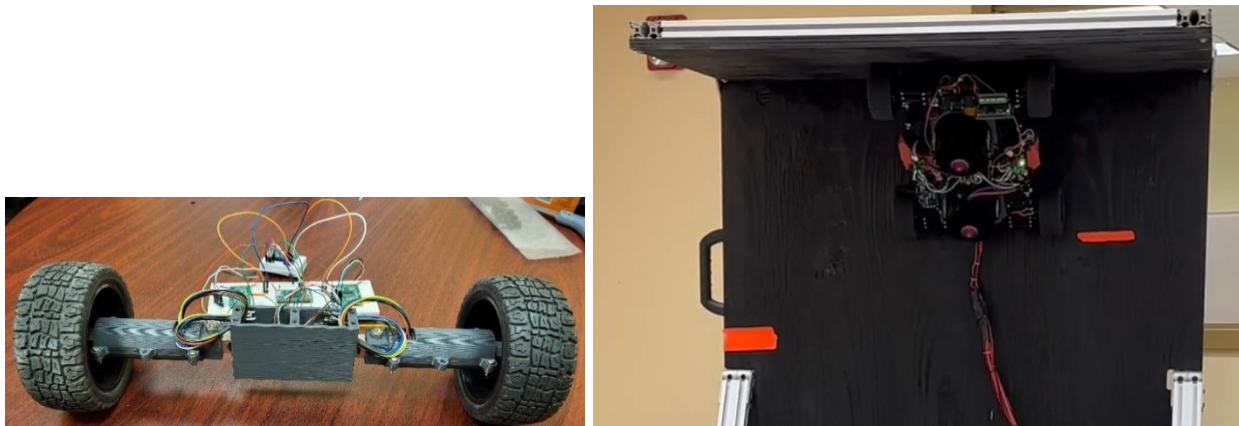
Figure 14. Assembly of load cell drive unit (left) and testing on dual-EDF platform (right).
