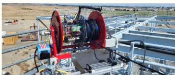
The "Lateral Gamma Scanner" crawler bot is lowered down the pipe and retracted using a reel and cable system.
