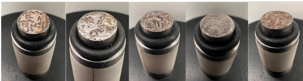
Figure 106. 6M caustic test results for the SRNL coupons (Coupons 1 through 5 - left to right).
