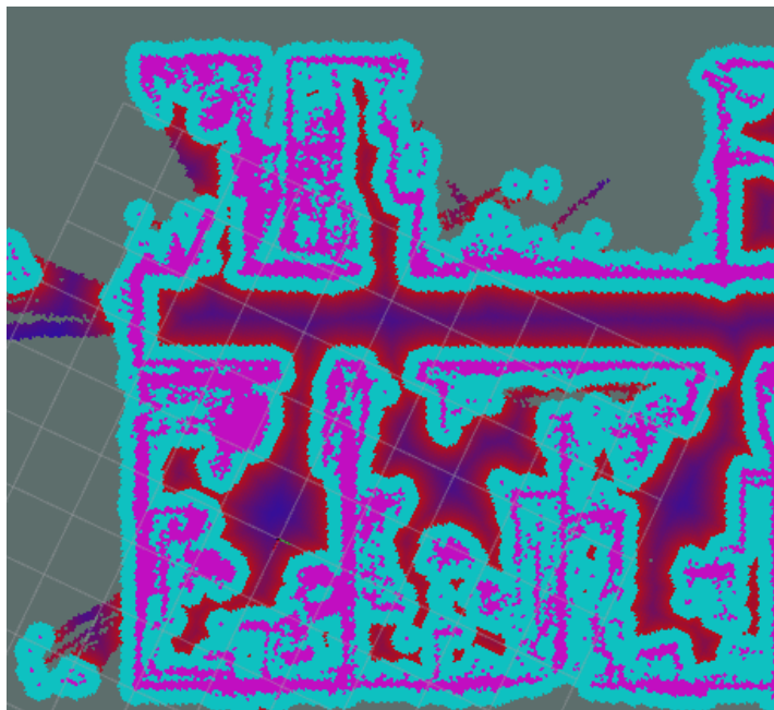
Figure 29. Partial costmap generated at a demonstration at Hanford CTF.
