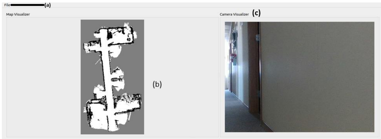
Figure 31. Menu bar (a), map (b), and camera visualizer (c) within the GUI.
