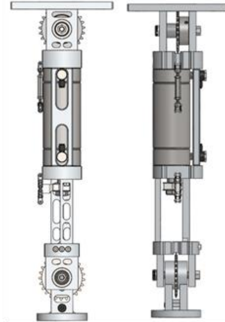
Figure 52. Front and side view joint of the Off-Riser Sampler System (ORSS).
