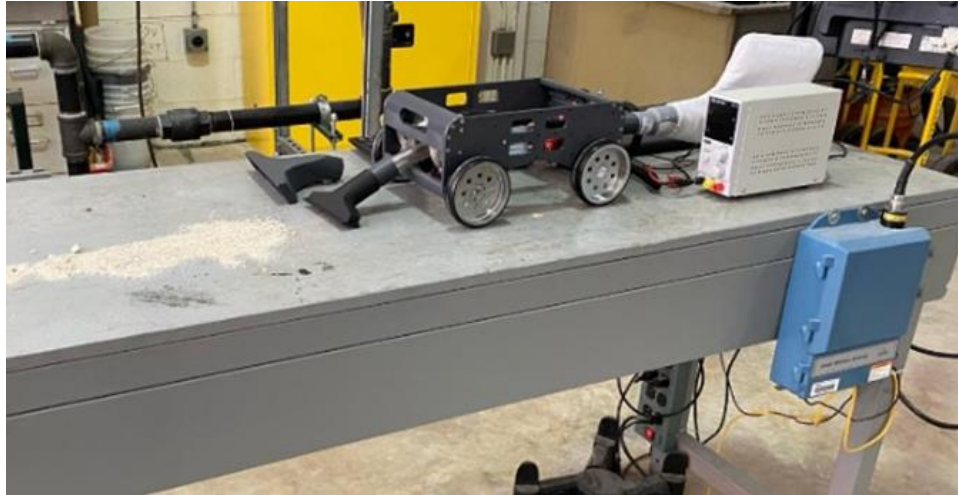
Figure 69. Testing the VCS's ability to vacuum similar gravel to that in the tank annulus.
