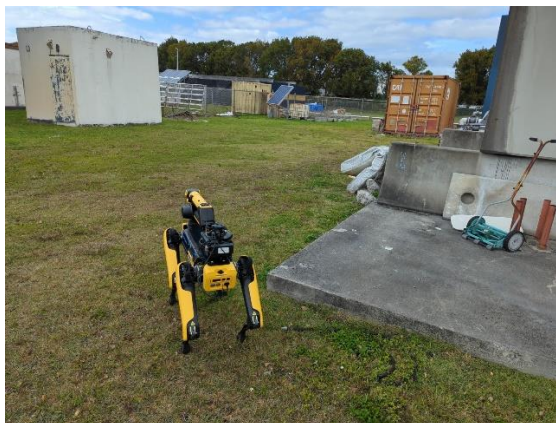
Figure 24. Spot platform autonomously navigating an unstructured outdoor environment.
