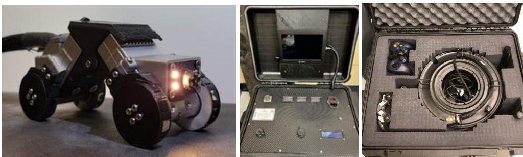
Figure 41. Deployed miniature inspection rover at AP-105 tank.
