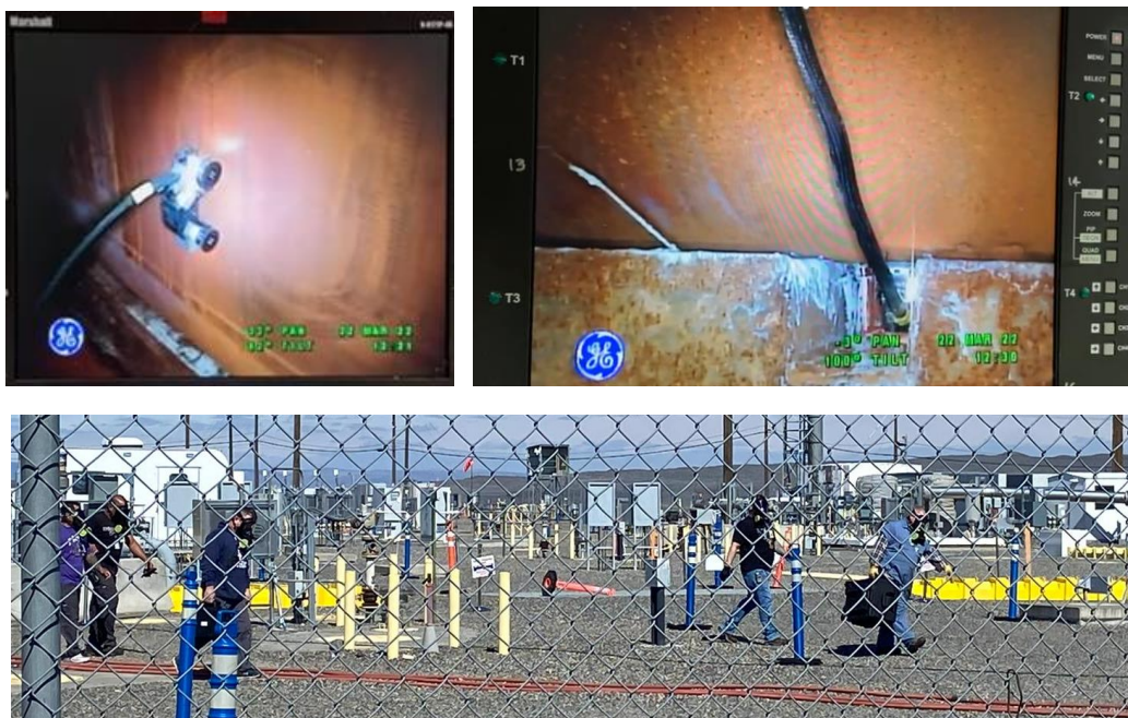
Figure 39. FIU's miniature inspection rover deployment at AP-105 DST.
