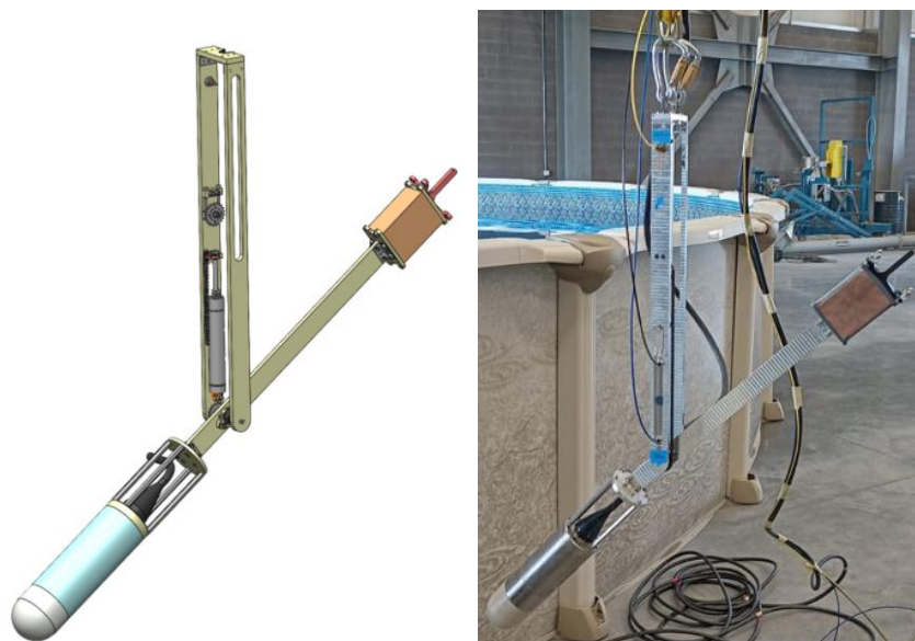
Figure 77. FIU's In-Tank Sonar System Prototype.
