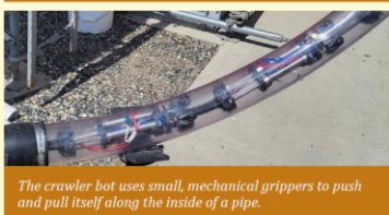
The crawler bot uses small, mechanical grippers to push and pull itself along the inside of a pipe.
