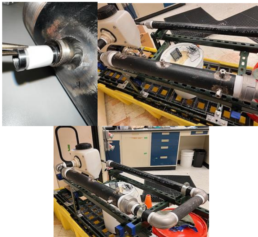
Figure 102. SRNL coupon assembly and loop testing.
