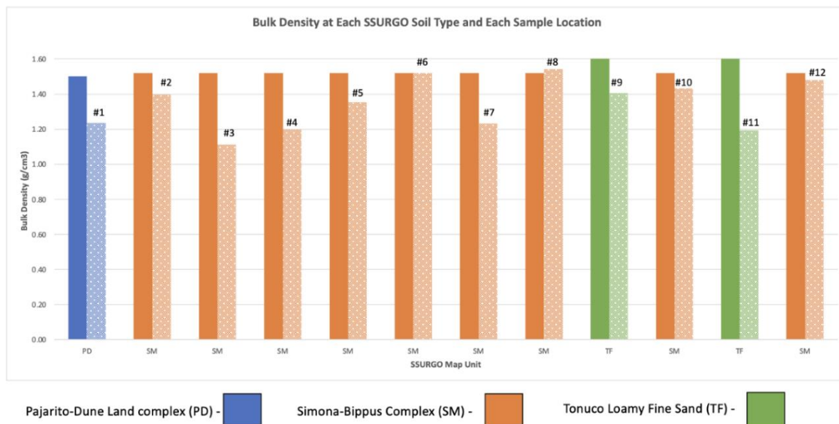
Figure 51. Graph of soil bulk density ( \text{g/cm}^3 ) for each SSURGO map unit and each soil sample location within these units.
