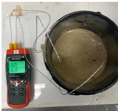
Figure 21. Initial testing of curing temperature of Endseal foam.
