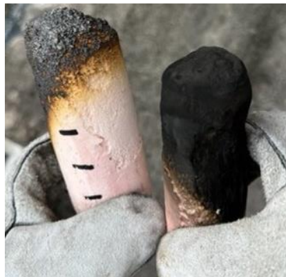
Figure 22. FoamBag TM flammability comparison with (left sample) and without (right sample) the Exolit AP-750 additive.
