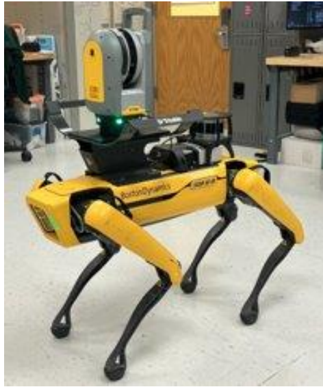
Figure 31. Finalized Spot/Trimble X7 complete payload configuration.
