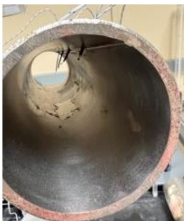
Figure 15. Pipe with thermocouples at varying depths.
