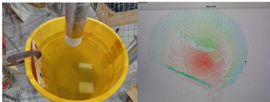
Figure 16. Objects inside 50-gallon Tank mimicking Hanford Tanks (left), sonar scan (right).
