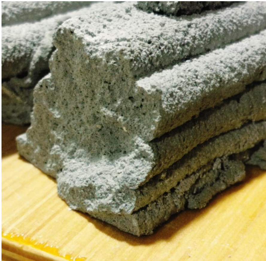
Figure 7. Fracture interface of 3D printed wall after 3 point bend test.
