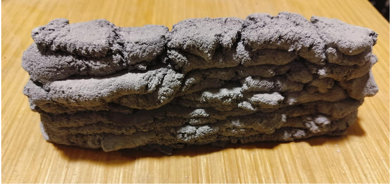
Figure 8. Poorly 3D printed wall due to unoptimized printable mixture.
