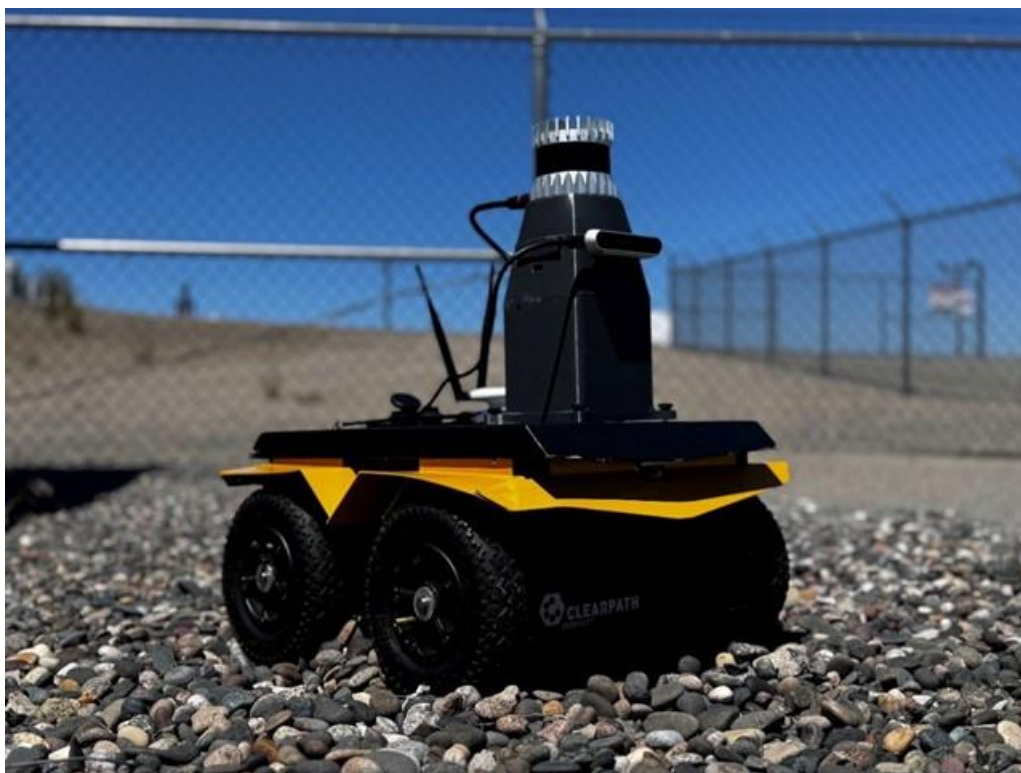
Figure 15. Clearpath Jackal equipped with a 3D Lidar, Depth Camera, and Wireless Telemetry at Hanford Cold Test Facility (CTF).
