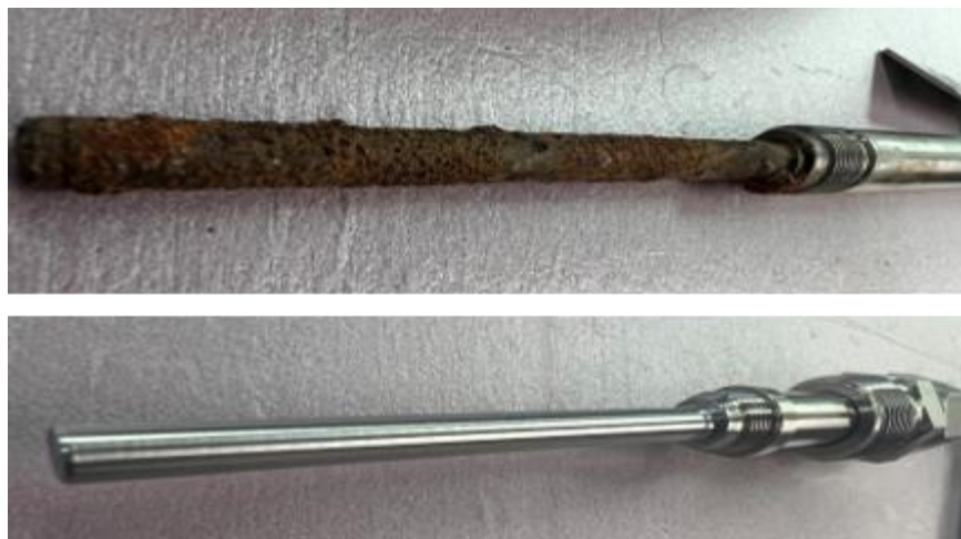
Figure 10. Carbon steel (ER) probes (bottom), before corrosion (top), and after corrosion.
