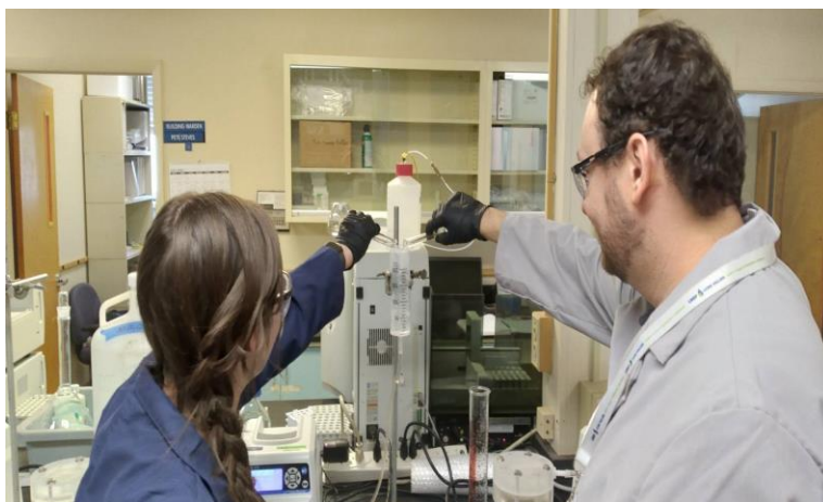
Figure 23. Valeria Ocampo (left) and Daniel Ohlson (Right) pouring in calcium citrate solutions and phosphate solutions simultaneously to ensure proper mixture of both solutions.
