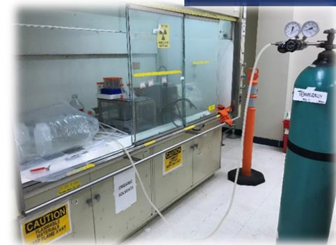
5% ammonia/95% nitrogen injection for montmorillonite long term U-aging experiment
