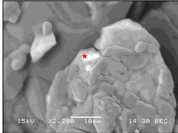
SEM image w/ EDS data for specimen 50-00A, prepared using a 50mM of \text{HCO}_3^- and 200ppm uranium pore water solution
