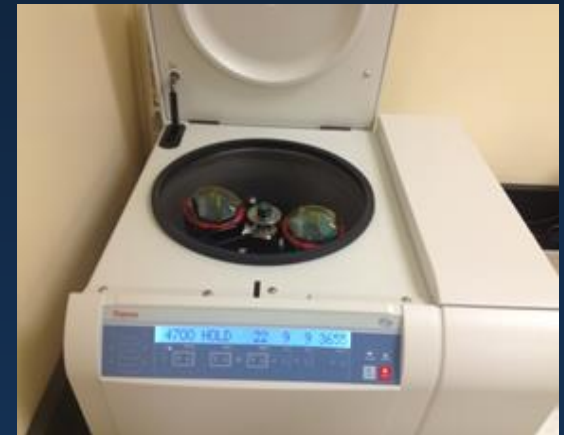
Centrifuge at 2700rpm (30min)
