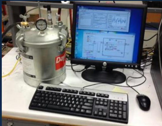
Isopiestic Vapor-Chamber connected to the acquisition system
