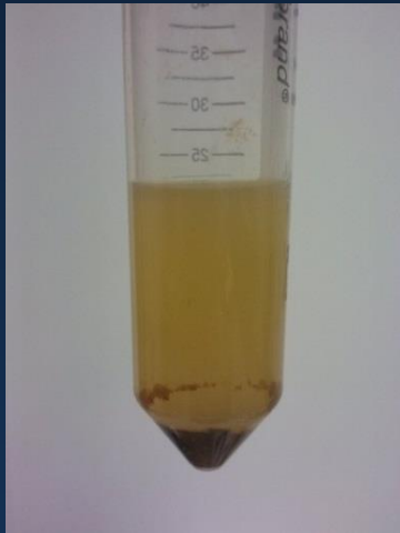
Centrifuge tube with sediment and humate solution
