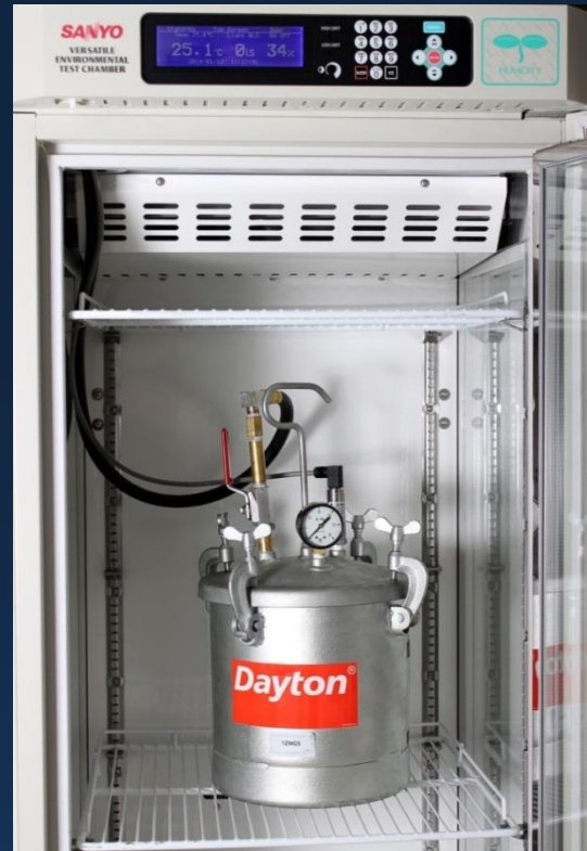
Isopiestic Vapor-Chamber connected to the acquisition system
