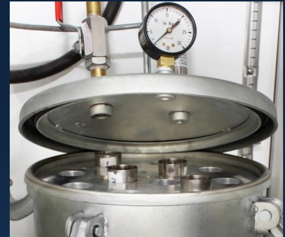
Aluminum block with holes for the nickel crucibles
