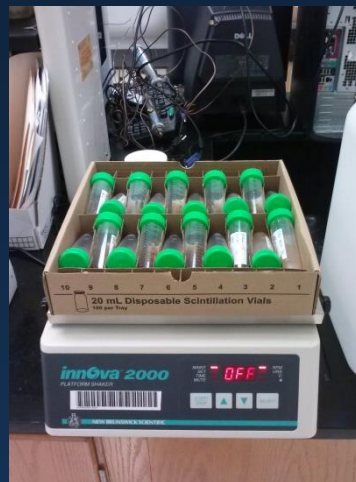
Samples in shaker table for 24 hours (100rpm)
