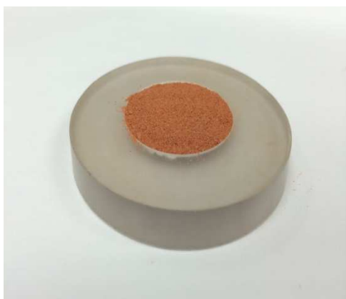
Figure 6. Amorphous sample holder with sediment to be placed into XRD instrument.
