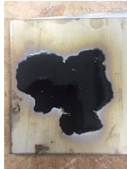
Significant discoloration, continued expansion and "off gassing", mass loss, desiccation, cracking, and brittle composition (500 degrees)
