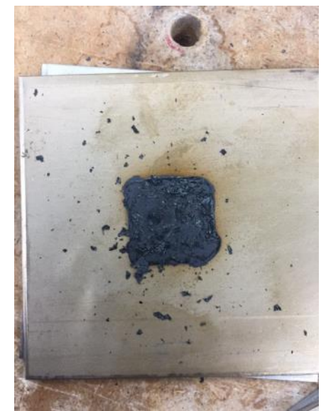
Significant mass loss, discoloration, desiccation, cracking, and flaking. Slightest abrasion with fixative resulted in total flaking. (800 degrees)
