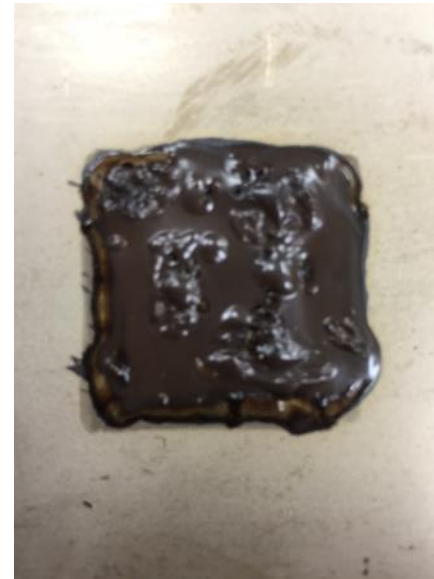
Significant discoloration, continued expansion, "off gassing", mass loss, desiccation, cracking, and brittle composition (500 degrees)
